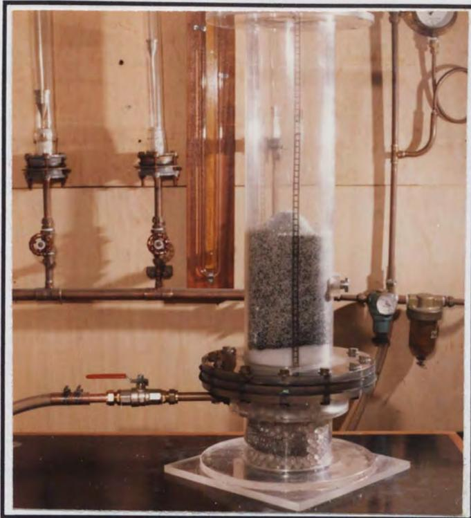
*Fig.10.62: Position of the flotsam band when started from "well mixed" state.*
