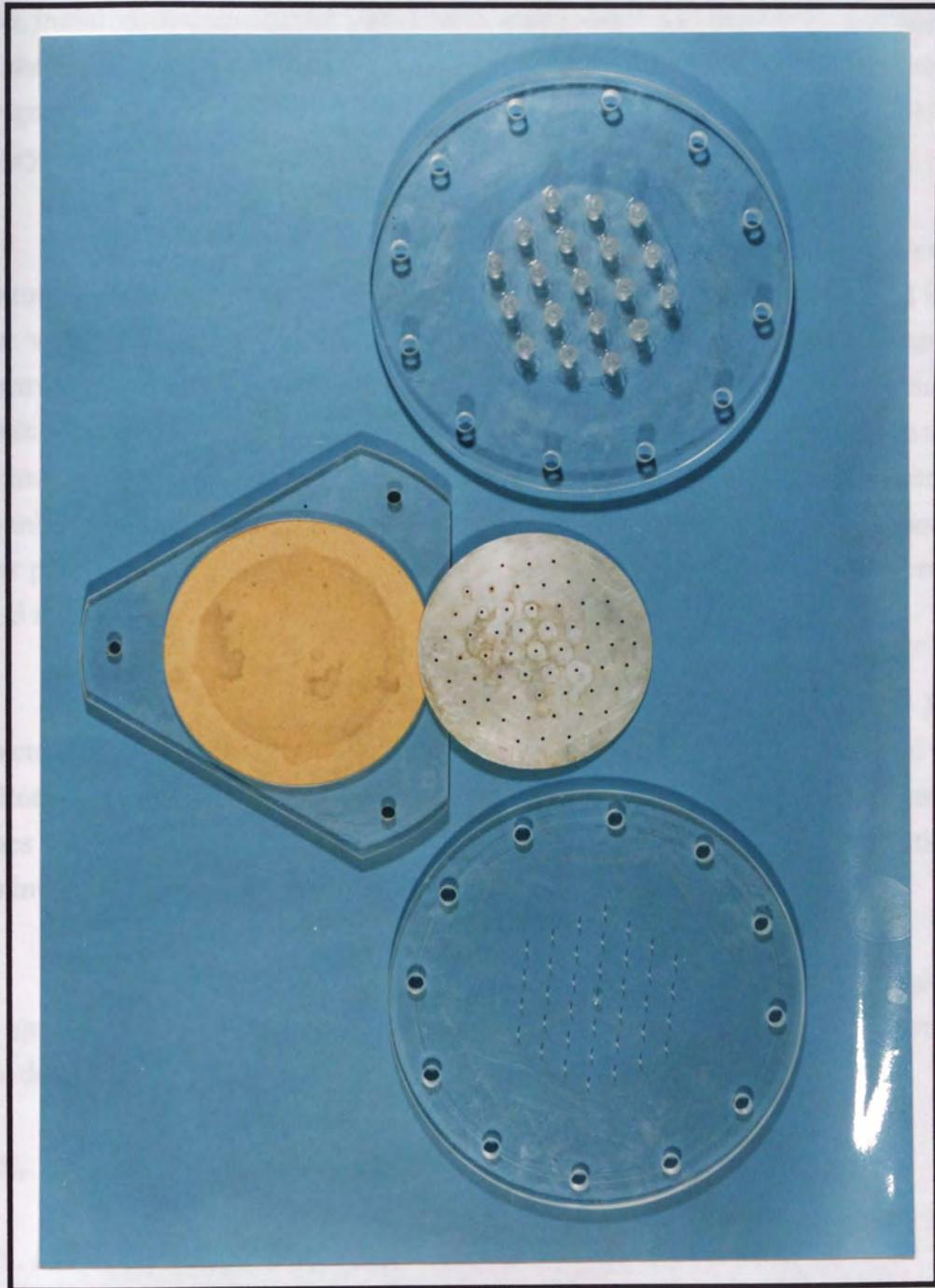
*Fig. 4.5: Photograph showing the distributors used in the fluidised bed systems*
