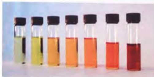
Figure 3: A photograph demonstrating that a range of CdSe NanoDots™ are capable of producing emissions over the entire visible spectrum
