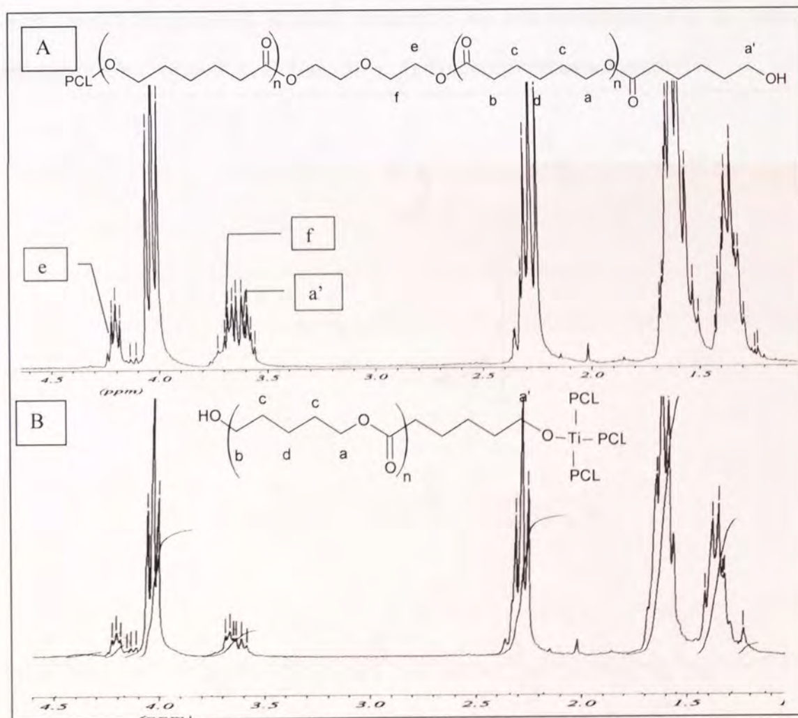
Figure 8.6: (A) ^1\text{H} NMR spectra of \text{PCL}_{1250} . (B) ^1\text{H} NMR spectra of product obtained from the poly-condensation of \text{Ti}(\text{O}-i\text{-Pr})_4 and \text{PCL}_{1250} .
