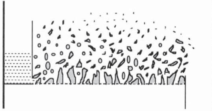
Figure 2.2 Schematic diagram of the biphasic dispersion in the spray regime.
