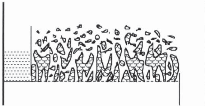
Figure 2.3 Schematic diagram of the biphasic dispersion in the mixed froth regime.
