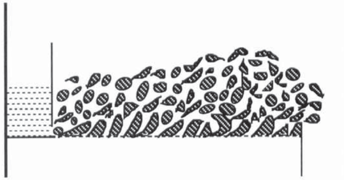
Figure 2.4 Schematic diagram of the biphasic dispersion in the emulsion flow regime.
