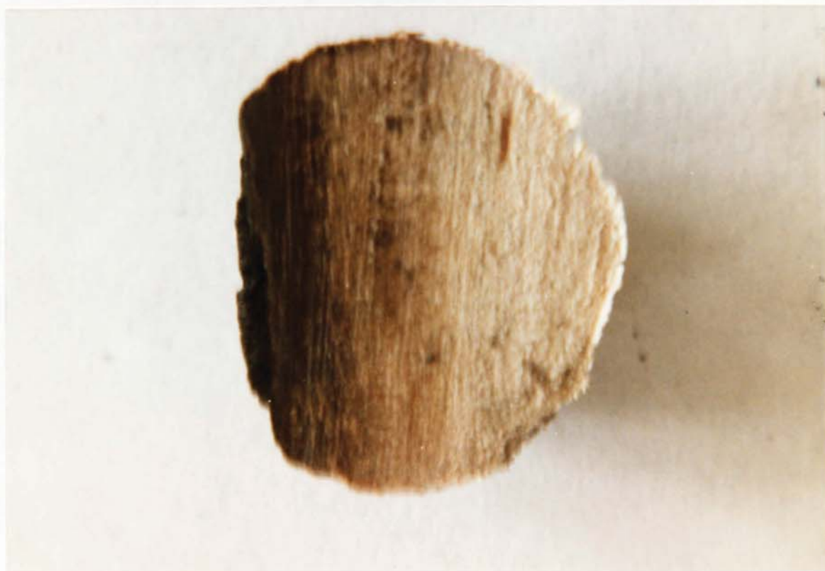
Plate 7.10 Section of Bead (5) Entering Flaming Pyrolysis Zone
