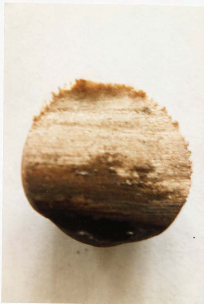
Plate 7.11 Section of Bead (6) Entering Flaming Pyrolysis Zone
