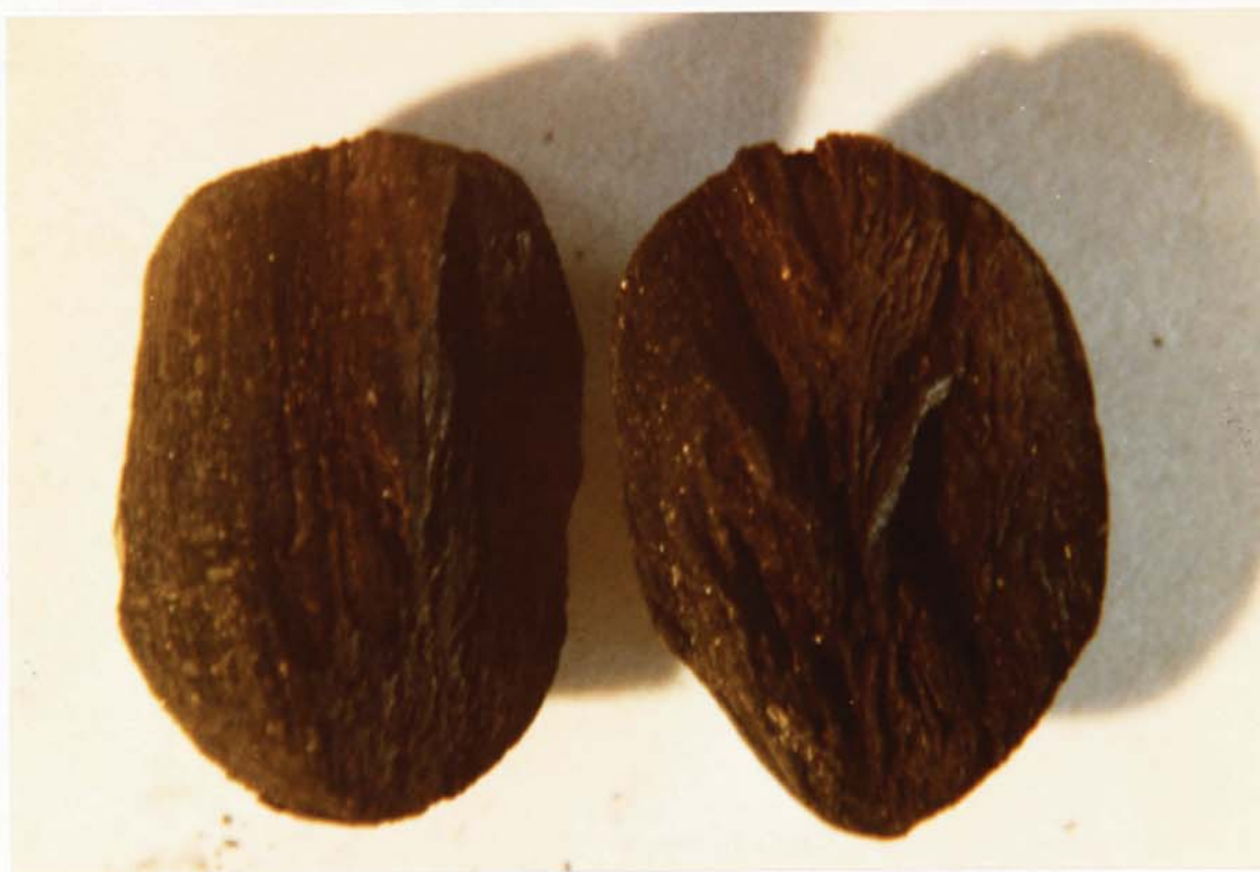
Plate 7.9 Split Charred Particle (2) Removed from Char Gasification Zone (Total Mass 0.54 g)
