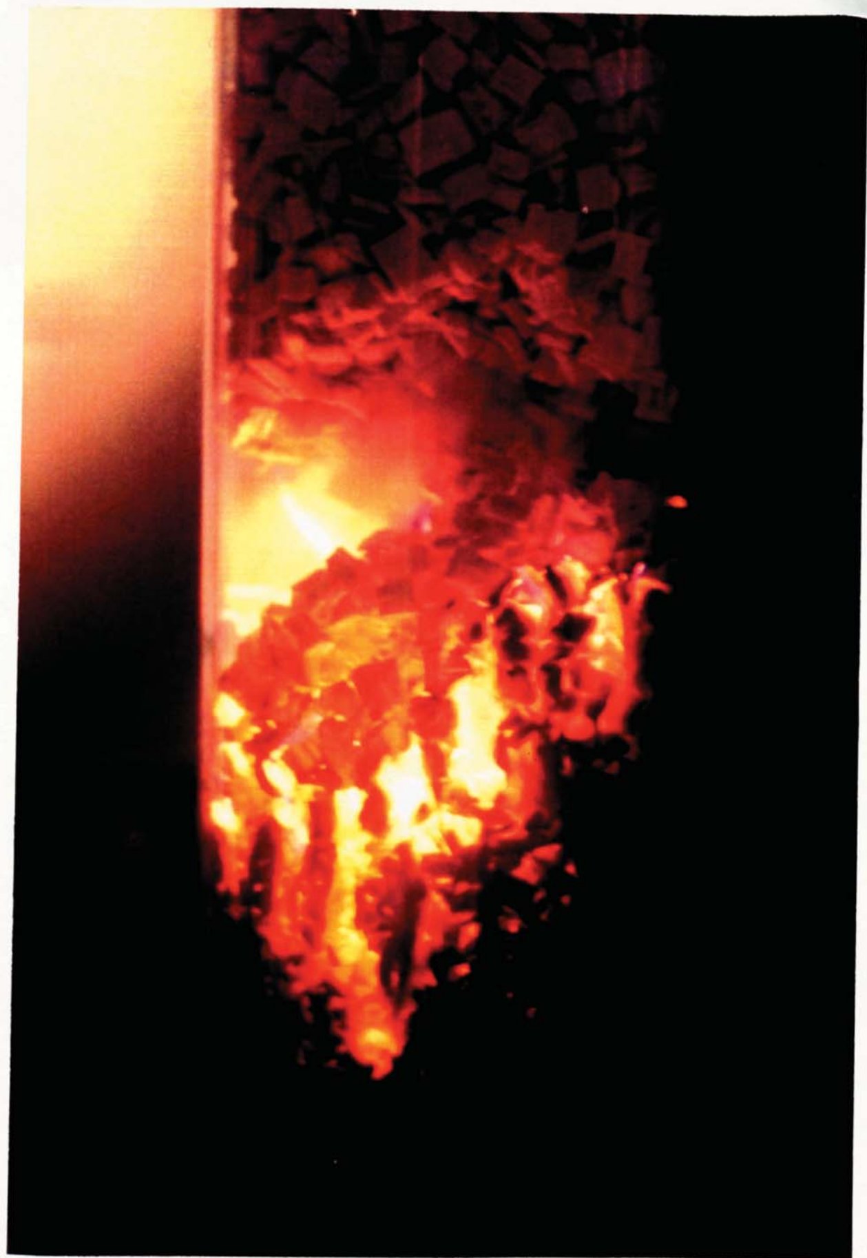
Plate 8.2 Feed Bridging in Gasifier (Experiment 7)
