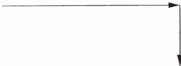
Figure 5.9 Connecting lines with an exit stream at a lower vertical position than the feed stream
