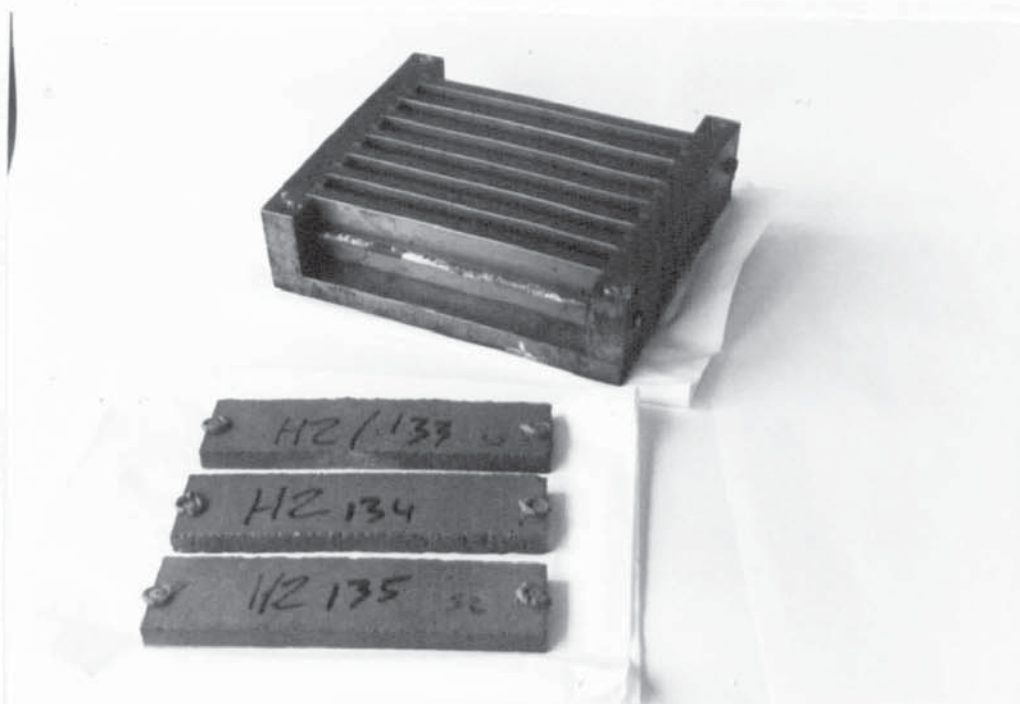
Fig 1.11 Mould and specimens produced for expansion studies.
