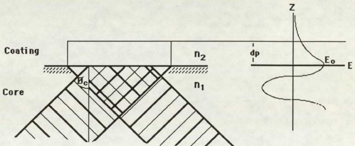
A standing sinusoidal wave is set up at the interface which penetrates the rarer medium, decaying exponentially. This is the evanescent wave and its penetration depth is given by the equation;
