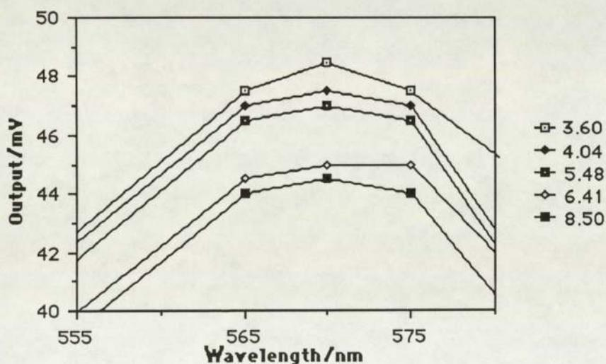
**FIG 5.8 Response Of Probe[(70:30) of (HEMA:MMA)] At 565nm**
