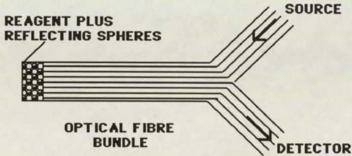
In order to reflect the modified incident light back towards the detector, small spheres are usually incorporated at the tip of the fibre close to or with the reagent phase. The second, configuration requires only a single fibre coupled with a beam splitter in order to separate the incident and emergent radiation; FIG 1.6
