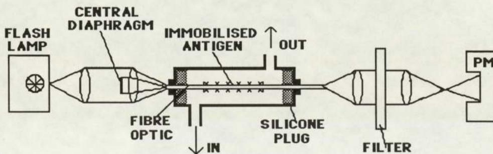
This was designed for the fluorescence detection of FITC labelled anti human IgG, when bound to immunologically immobilised antigen at a glass-liquid interface. This device uses the evanescent wave component of the incident light as the excitation wavelength and the associated excited wavelength as the signal picked up by the fibre optic. A similar device using fluorophores immobilised in lipid membranes is described in the literature<sup>100,101</sup>.
