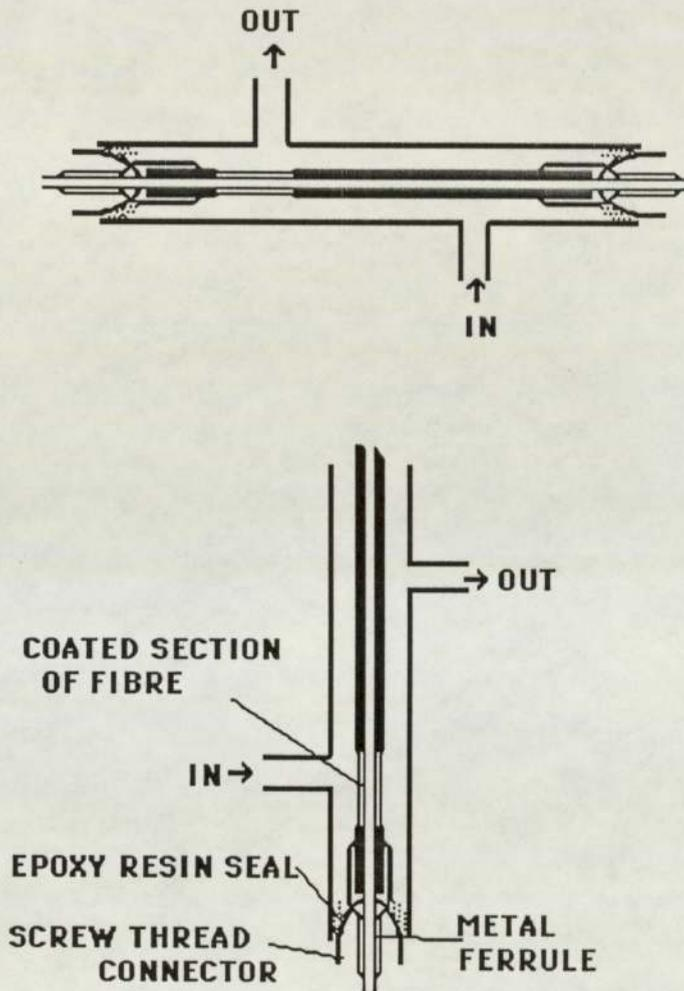
The fact that the cell had to be screwed into place at both ends presented problems with the opposite twisting action of the connections and this, combined with the fact that the cells were made of glass created further problems with their inherent fragility. The cells were not water tight and solution leaked into the bulk head causing the optical interface between fibres to change. This problem was temporarily lessened by standing the cell vertically and only gluing a ferrule at the
