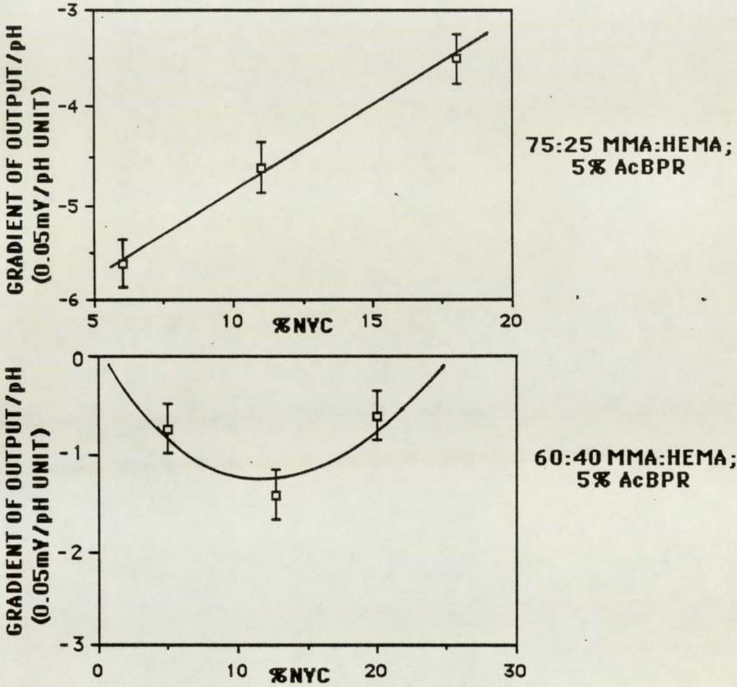
FIG 7.8 Effect On Response Gradient Of Ratio HEMA:MMA:5%NYC
