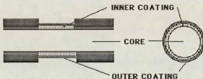
The inner and outer layer contained encapsulated reagent in some cases and the outer layer was reagent free in others as described in TABLE 5.2.
