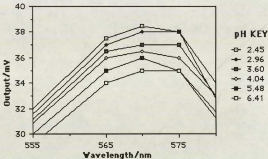
**FIG 5.6 Response of Probe [(70:30):5% of (HEMA:MMA):AcBPR] at 565nm to Changing pH**
