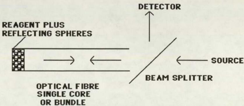
The incident or background light may need to be distinguished from the signal travelling along the fibre, towards the detector. In the case of a fluorescent reagent, this
