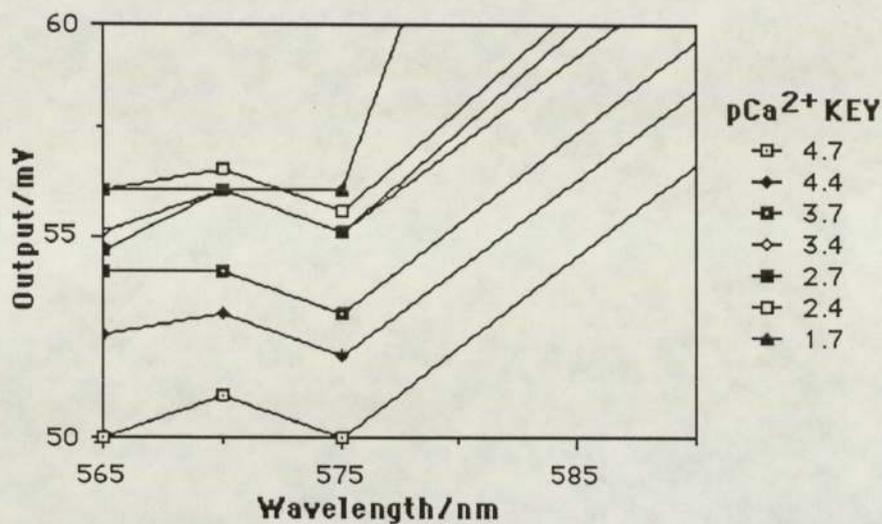
FIG 5.10 Response Of Probe [(70:30):5% of (HEMA:MMA):AcBPR] To Calcium Chloride At 565nm
