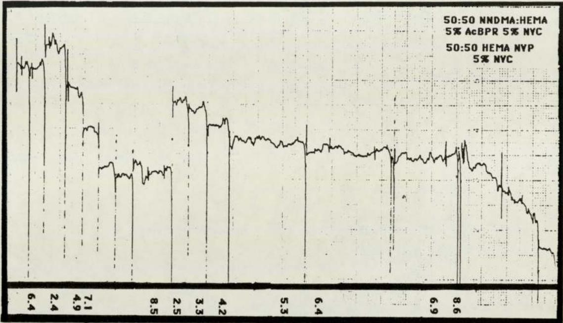
**FIG 5.13 Response Of Probe Without High Water Content Exterior Layer.**
