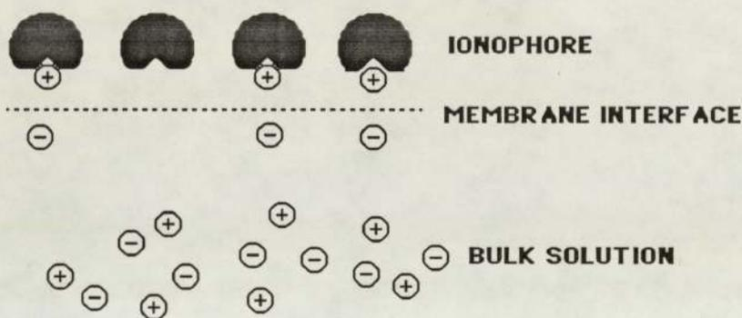
Ionophores, such as valinomycin, have electron rich pockets, which selectively extract those cations which will fit into the pockets, leaving the co-anions behind in the bulk solution and thus creating a charge separation at the membrane/solution interface. The trans-membrane potential, thus generated, is proportional to the log of the analyte activity and for ideal Nernstian behaviour is given by the equation<sup>3</sup>:-
