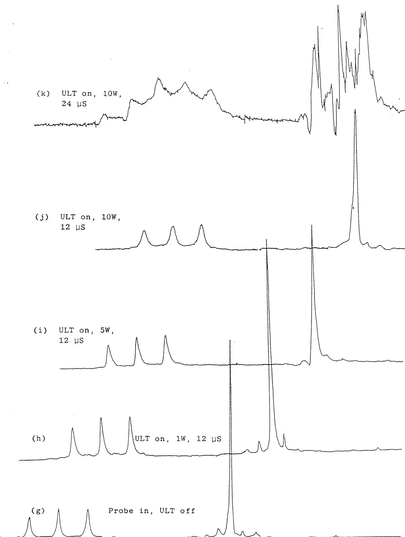
Figure 8.10 (g)-(h): The effects of ultrasound at a frequency of 6MHz on proton NMR signals observed for a saturated solution ammonium chloride in deuterated dimethylsulfoxide containing a trace of hydrochloric acid. The effects shown are for applying increasing power ranging from 1W to 10W across the transducer and changing the NMR pulse width (us).
