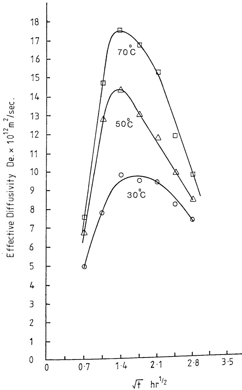
Figure 9.16 Variation of effective diffusivity for n-hexadecane with adsorption time at temperatures 303, 323 and 343°K
