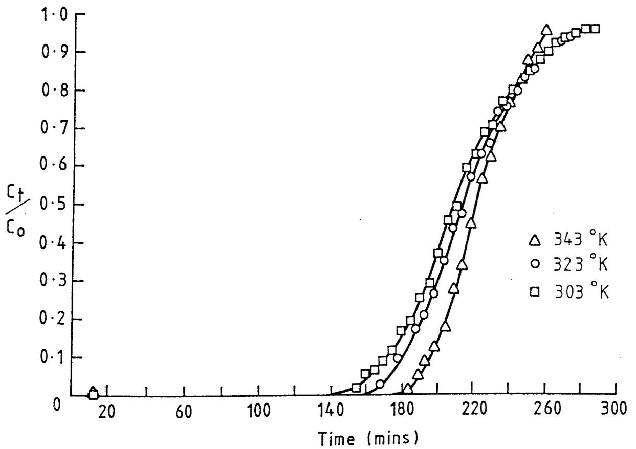
Figure 9.20 Effect of temperature on breakthrough curve of n-dodecane
