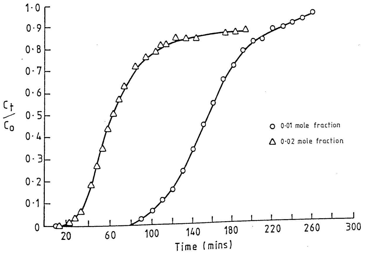
Figure 9.27 Effect of feed concentration on breakthrough curve of n-hexadecane
