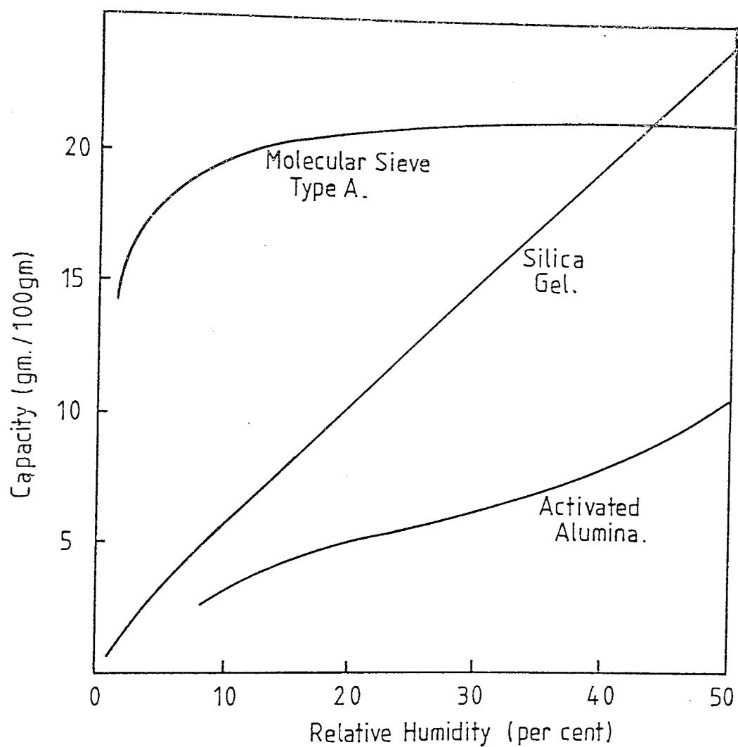
Figure 3.3 Water vapour adsorption on different adsorbents at 25°C
