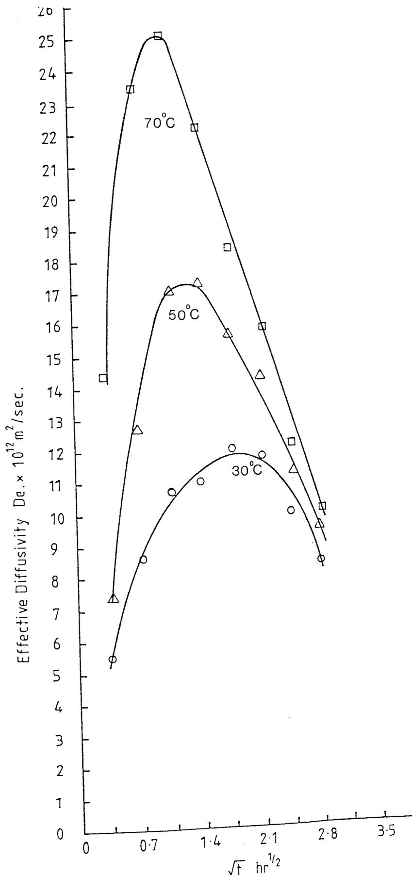
Figure 9.15 Variation of effective diffusivity for n-dodecane with adsorption time at temperatures 303, 323 and 343°K
