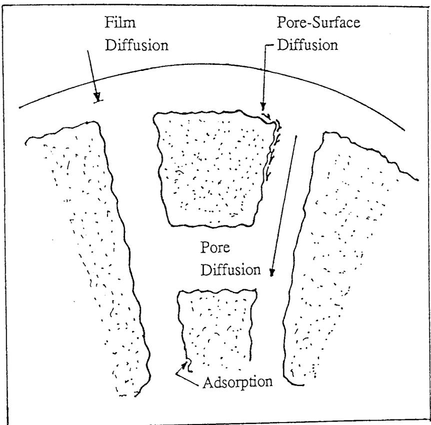
Figure 4.2 Adsorption on a porous adsorbent particle
