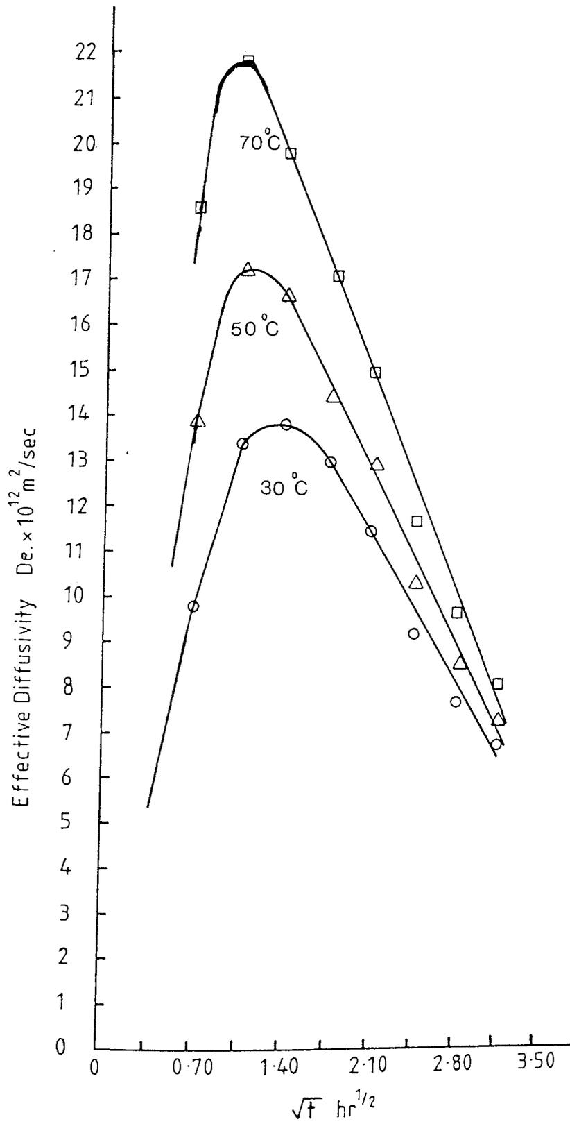
Figure 9.17 Variation of effective diffusivity for n-eicosane with adsorption time at temperatures 303, 323 and 343°K
