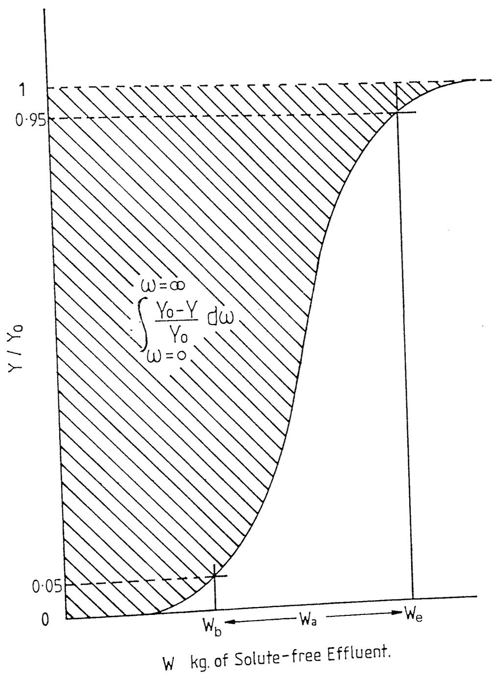
Figure 5.2 Breakthrough curve used in determination of total dynamic capacity
