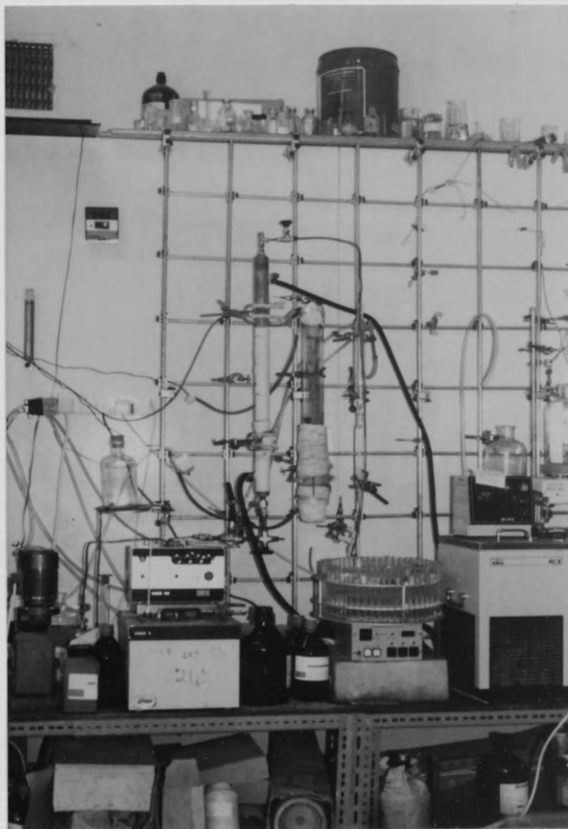
Figure 7.5 General arrangement of dynamic adsorption apparatus
