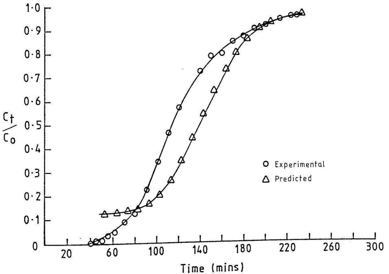
Figure 9.41 Experimental and Predicted breakthrough curves using the derived model, for adsorption of n-icosane with type 5A molecular sieves in Run 23
