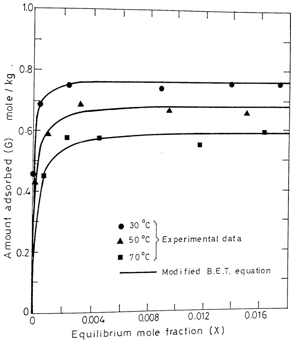
Figure 9-1: Adsorption isotherms of n-dodecane
