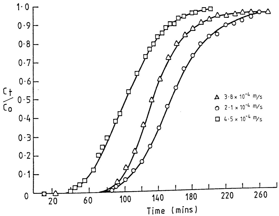
Figure 9.30 Effect of superficial velocity on breakthrough curve of n-hexadecane
