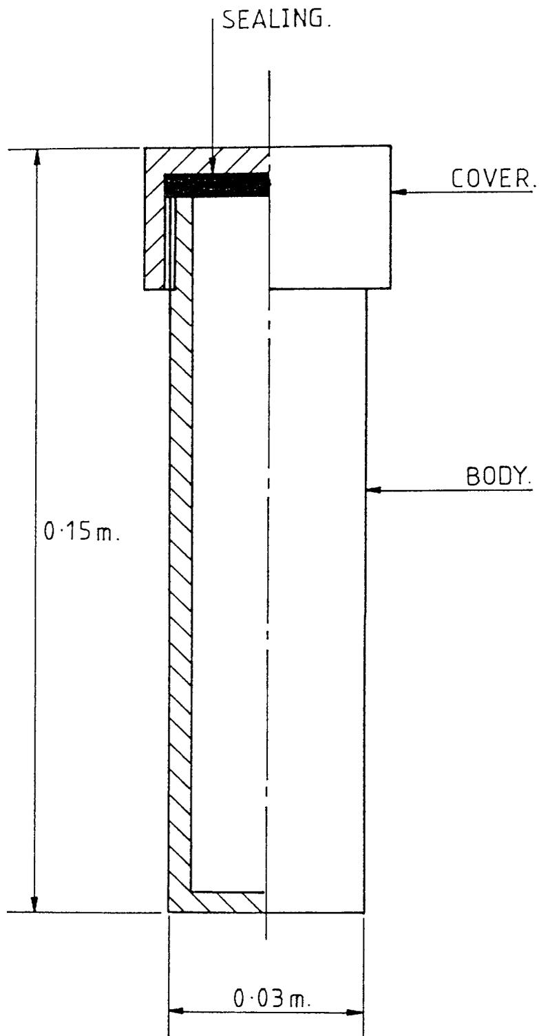
Figure 7.1 Batch adsorption tube
