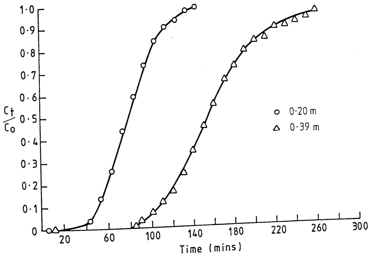
Figure 9.24 Effect of bed height on breakthrough curve of n-hexadecane
