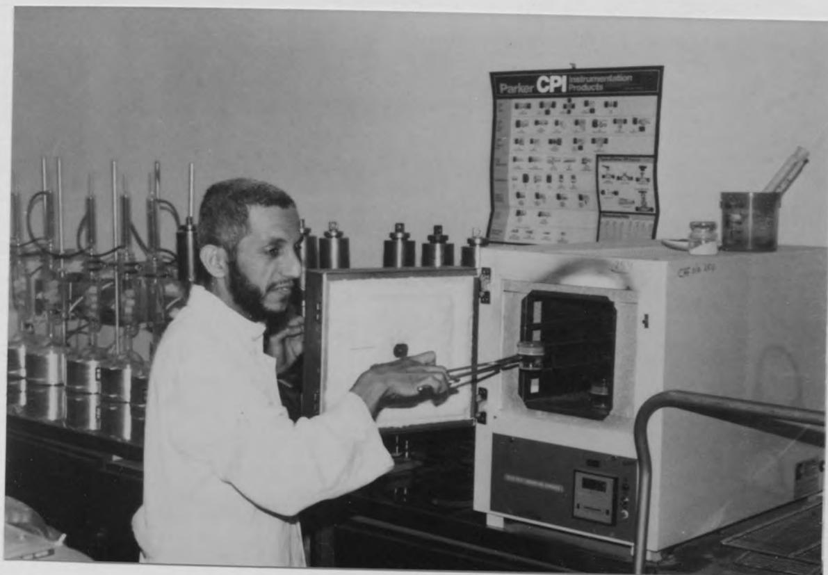
Figure 7.3    Activation of molecular sieves for batch experiments
