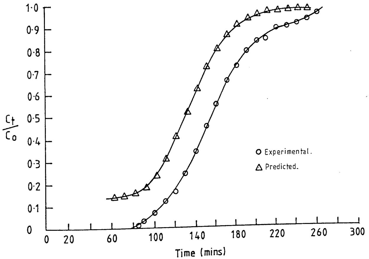
Figure 9.40 Experimental and Predicted breakthrough curves using the derived model, for adsorption of n-hexadecane with type 5A molecular sieves in Run 15
