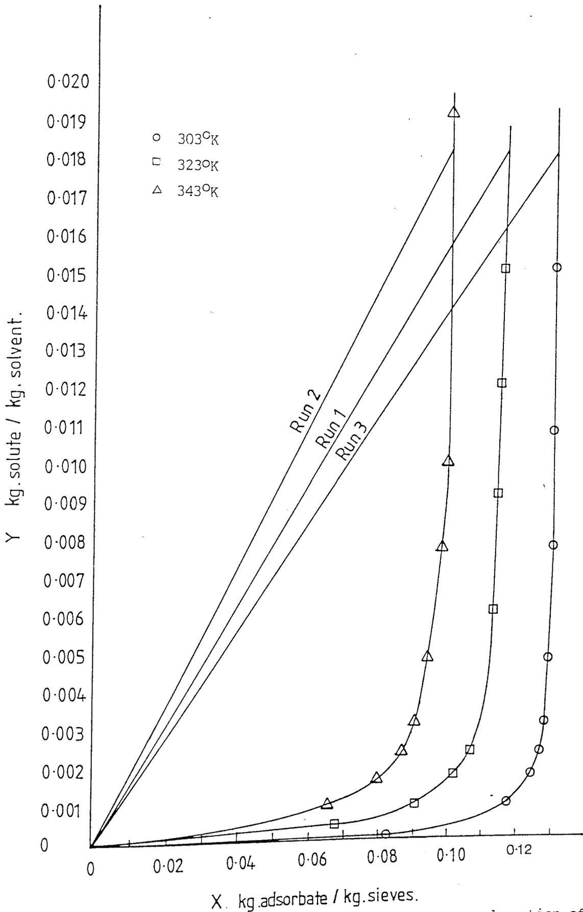
Figure B.5 Equilibrium curves and operating lines for adsorption of n-dodecane
