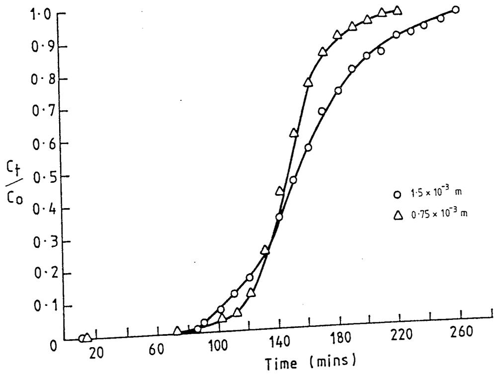
Figure 9.32 Effect of particle size (average diameter  $d_p$ ) on breakthrough curve of n-hexadecane
