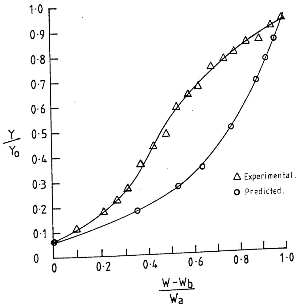
Figure 9.36 Comparison between experimental and predicted curves using Treybal's method (42) for adsorption of n-dodecane at 323°K with Type 5A molecular sieves
