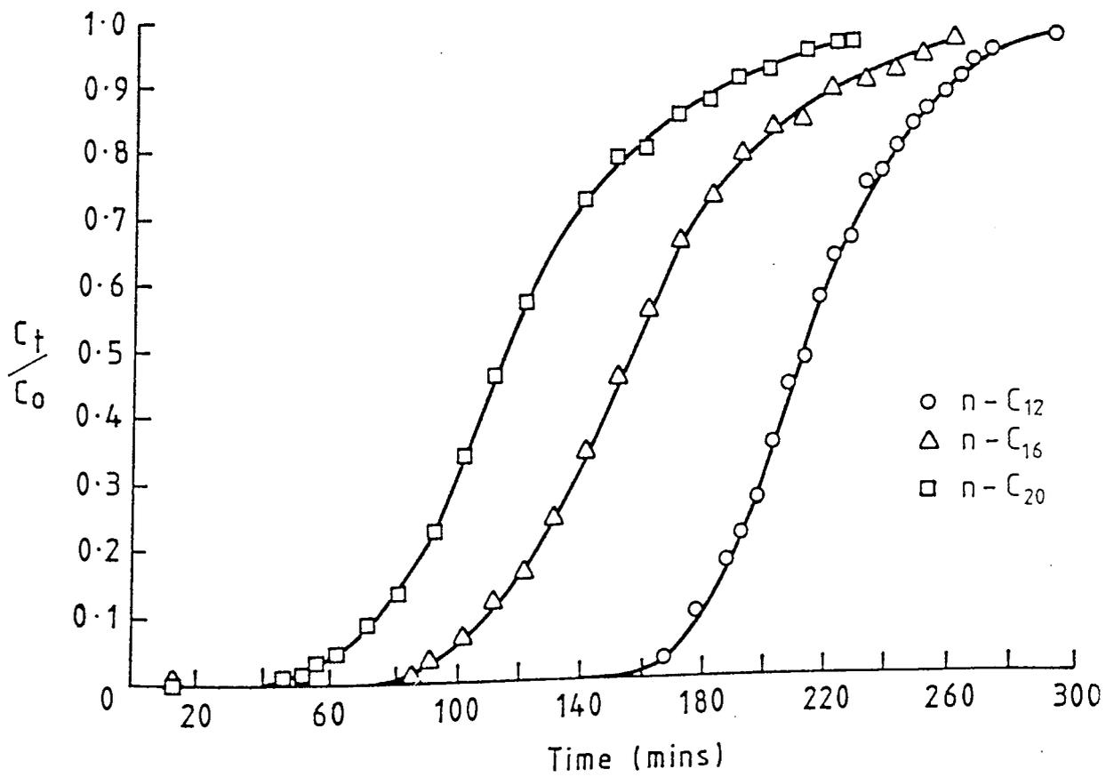
Figure 9.19 Breakthrough curves of n-paraffins at 323°K
