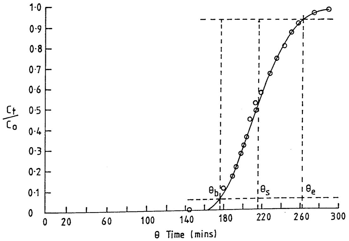
Figure 9.18 Experimental breakthrough curve
