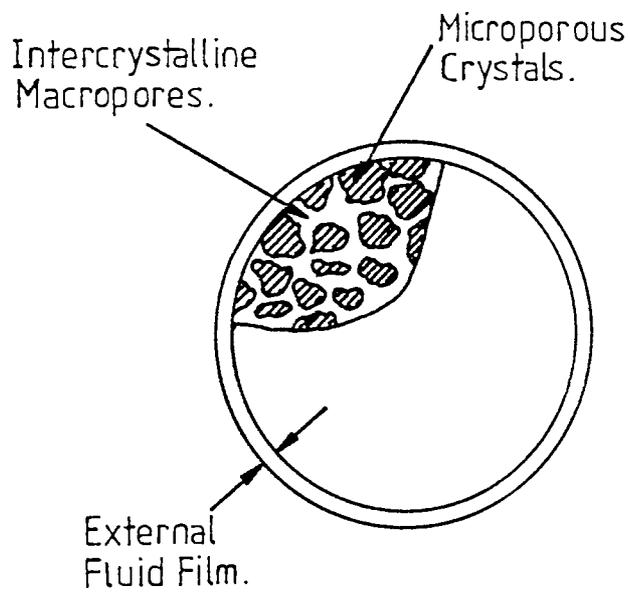
Figure 5.4 Schematic diagram of composite adsorbent pellet showing the three principal resistances to mass transfer
