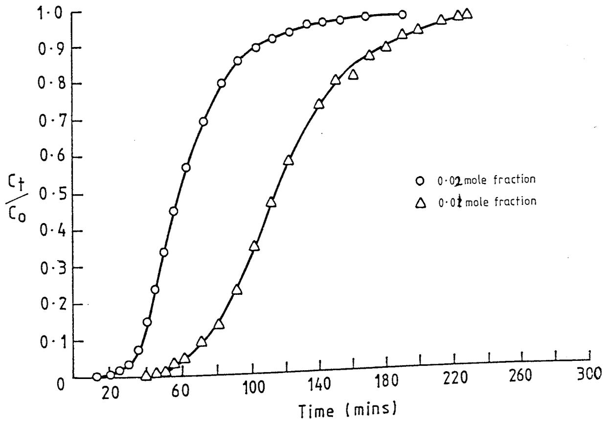
Figure 9.28 Effect of feed concentration on breakthrough curve of n-icosane
