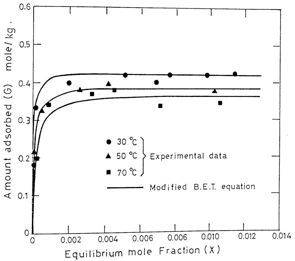
Figure 9.2: Adsorption isotherms of n-hexadecane
