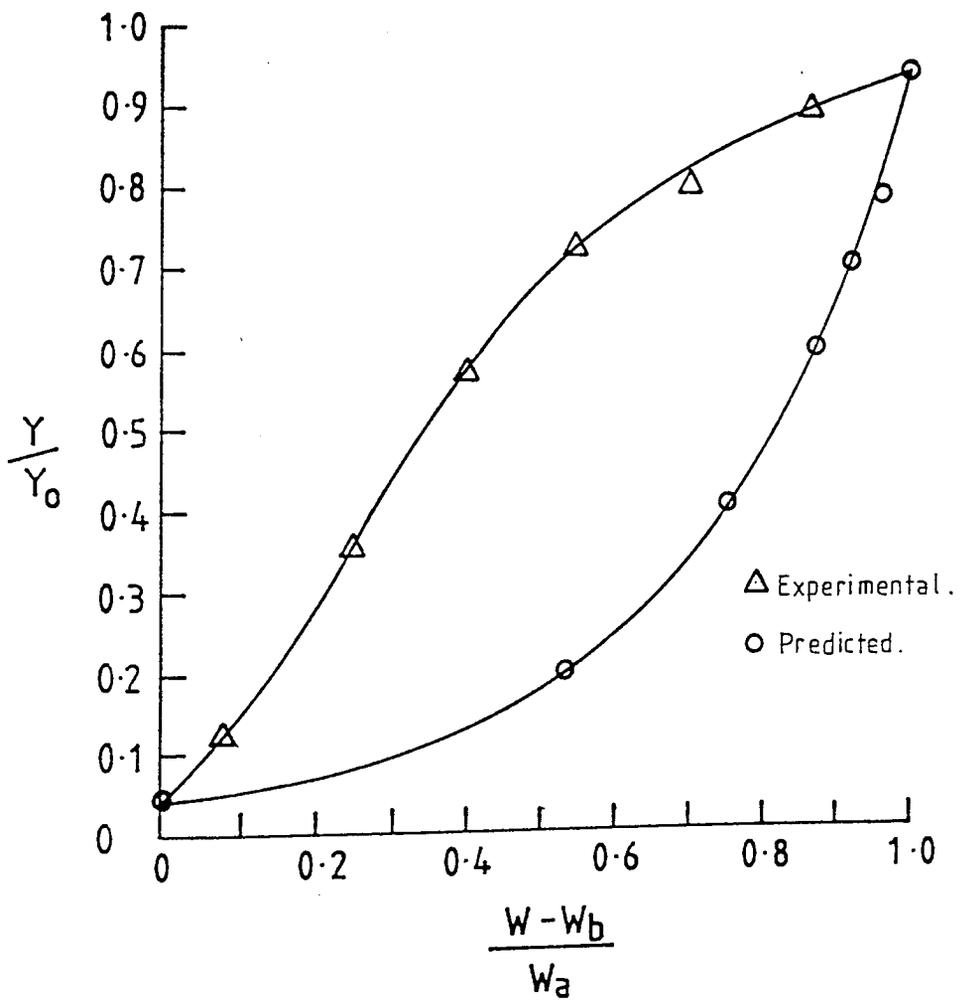
Figure 9.38 Comparison between experimental and predicted curves, using Treybals method (42) for adsorption of n-hexadecane at 323°K with type 5A molecular sieves
