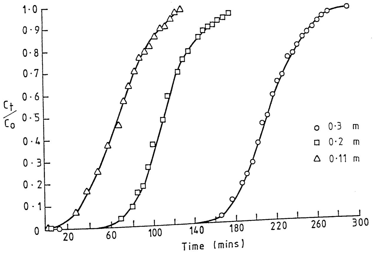
Figure 9.23 Effect of bed height on breakthrough curve of n-dodecane
