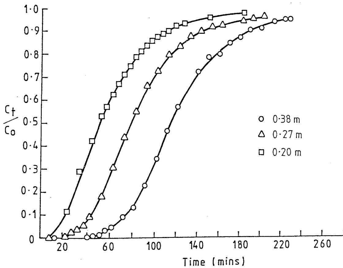
Figure 9.25 Effect of bed height on breakthrough curve of n-eicosane
