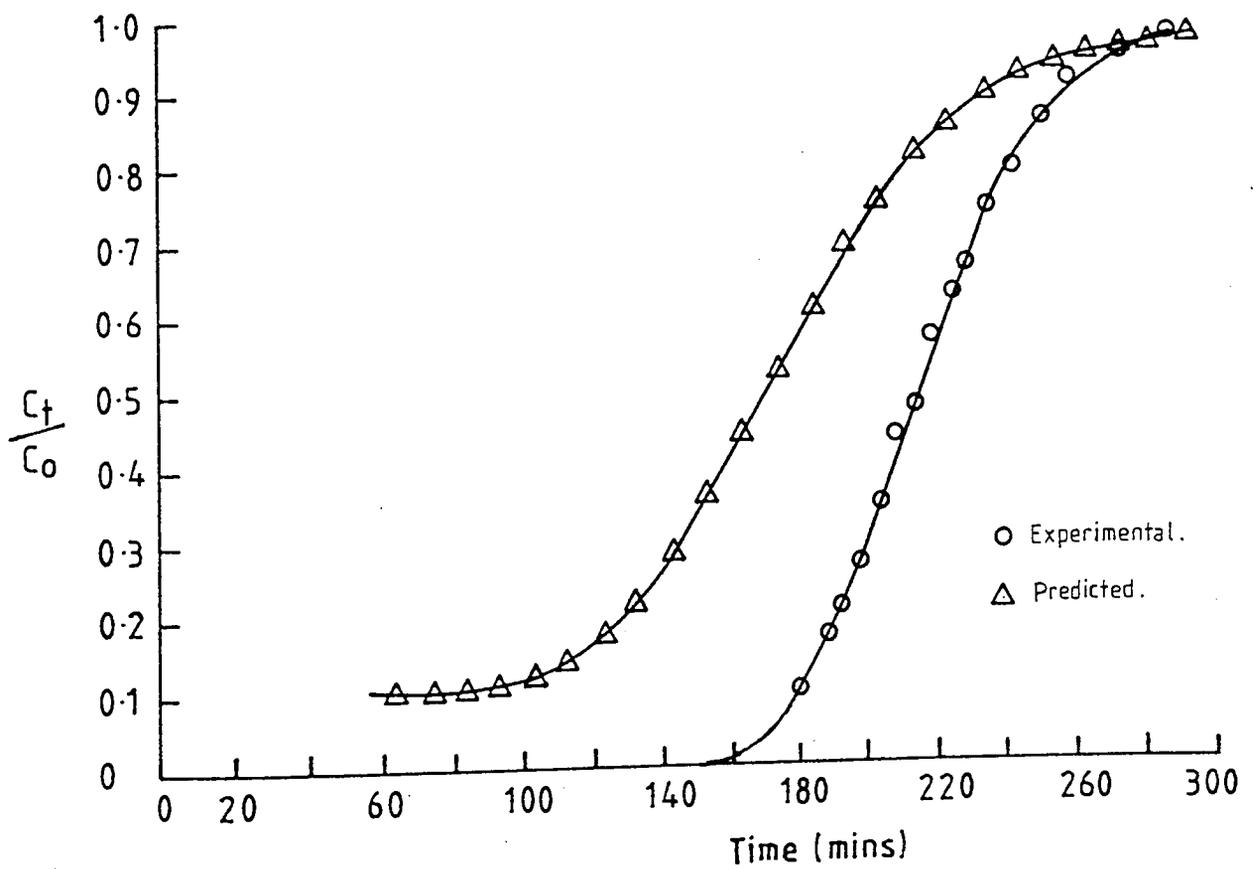
Figure 9.39 Experimental and Predicted breakthrough curves using the derived model, for adsorption of n-dodecane with type 5A molecular sieves in Run 1
