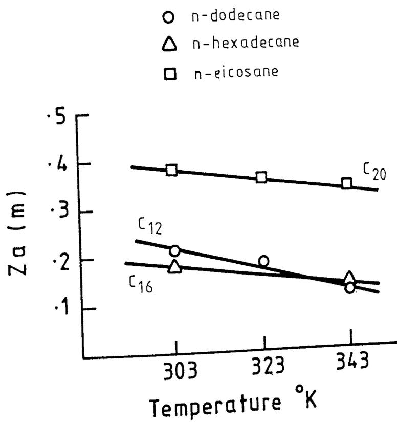
Figure 9.35 Effect of temperature on adsorption zone height
