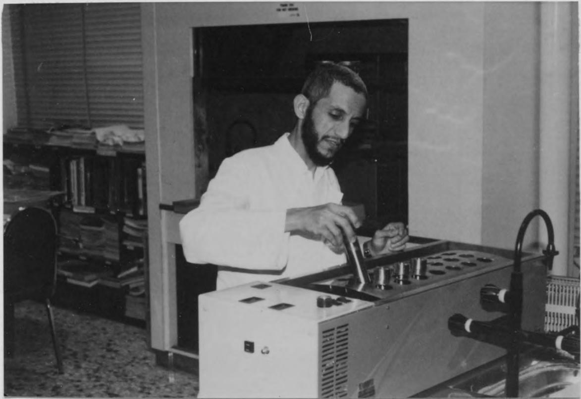
Figure 7.2 Thermostatic water bath for batch experiments
