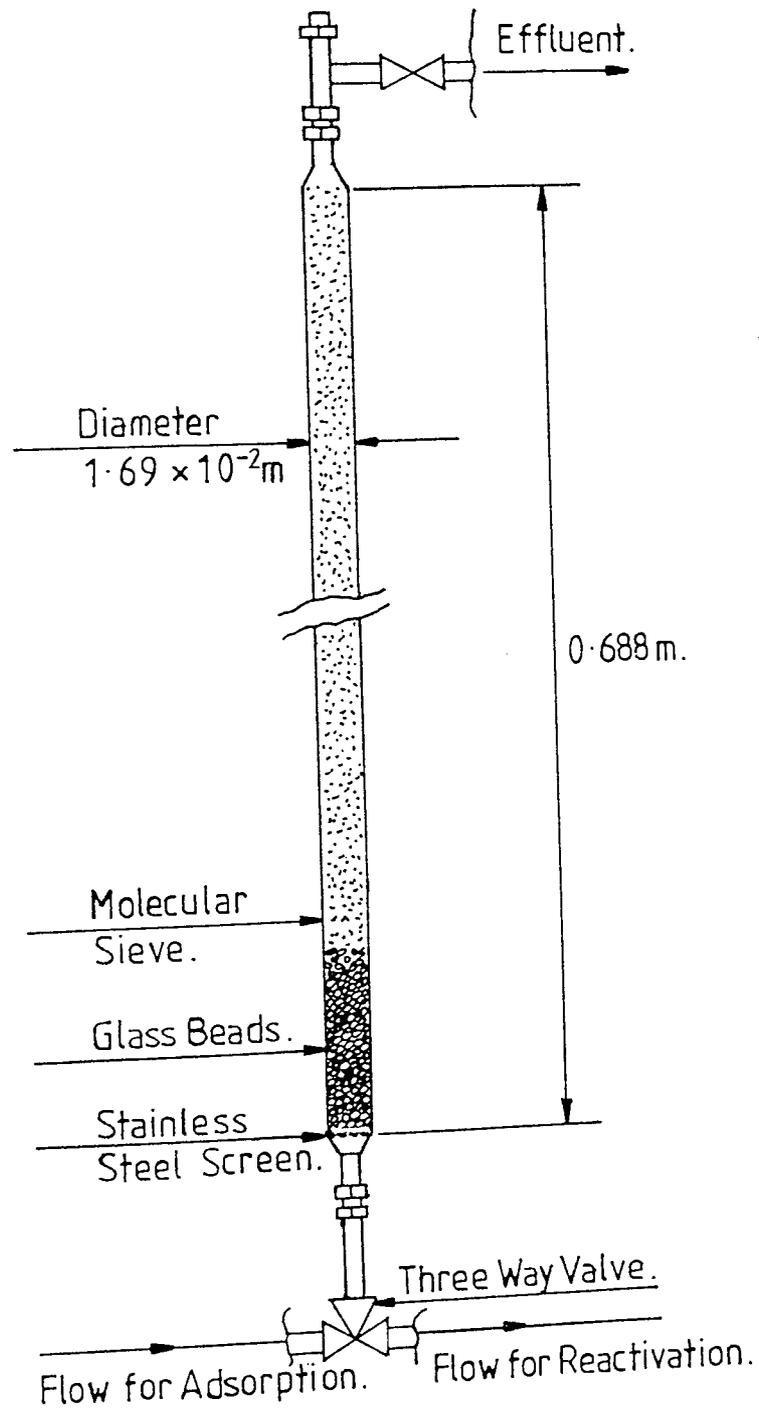
Figure 7.8 Adsorption column
