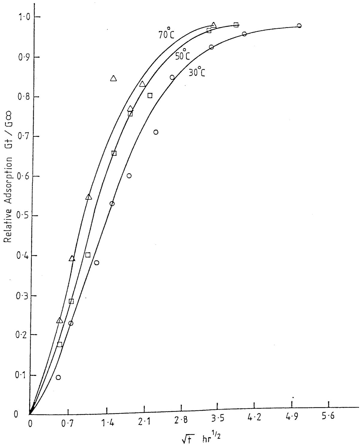
Figure 9.9 Kinetics of adsorption of n-dodecane from isooctane solutions at various temperatures
