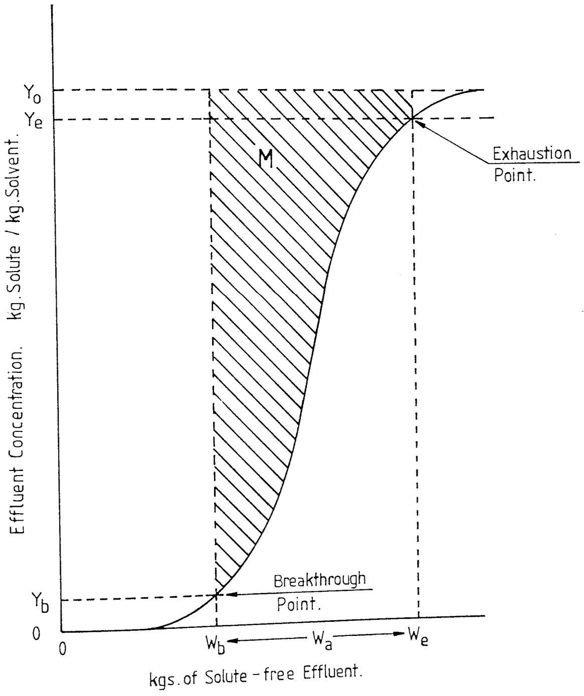
Figure 5.1 Idealised breakthrough curve
