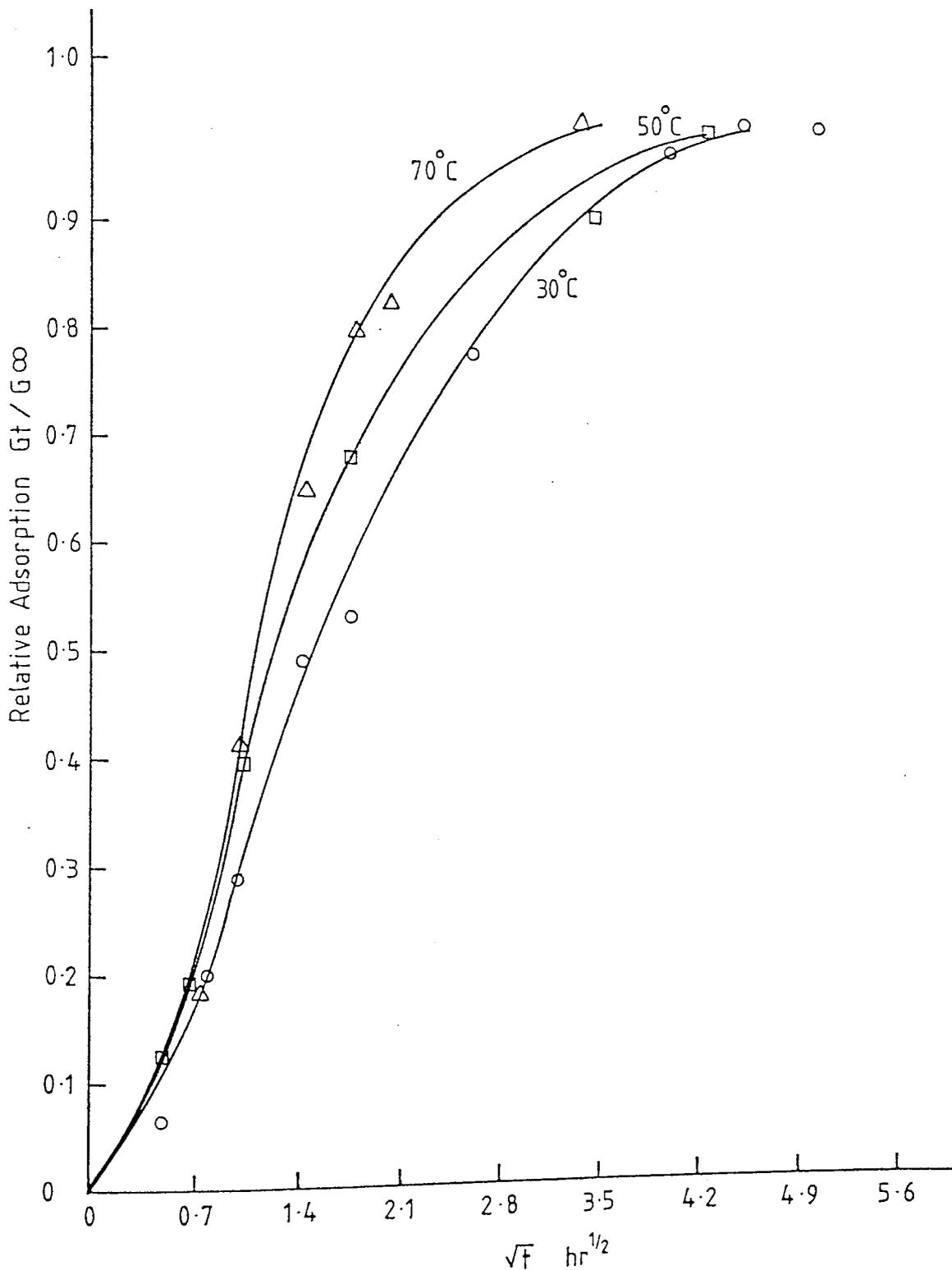
Figure 9.10 Kinetics of adsorption of n-hexadecane from isooctane solution at various temperatures
