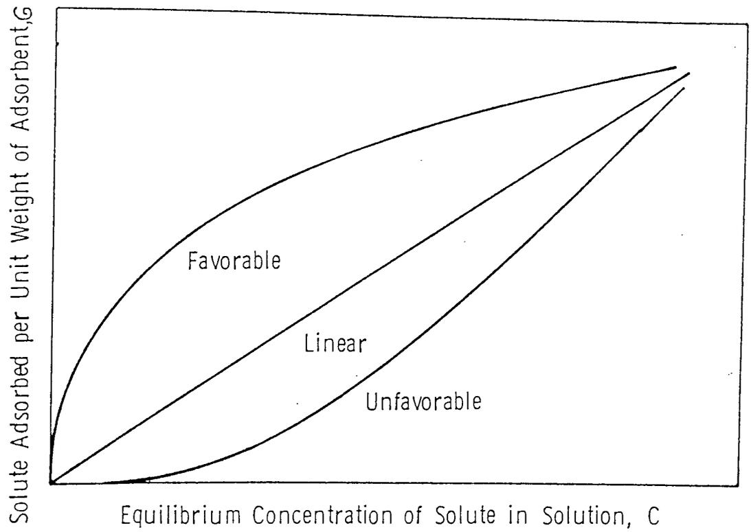
Figure 4.1. Basic types of adsorption isotherms
