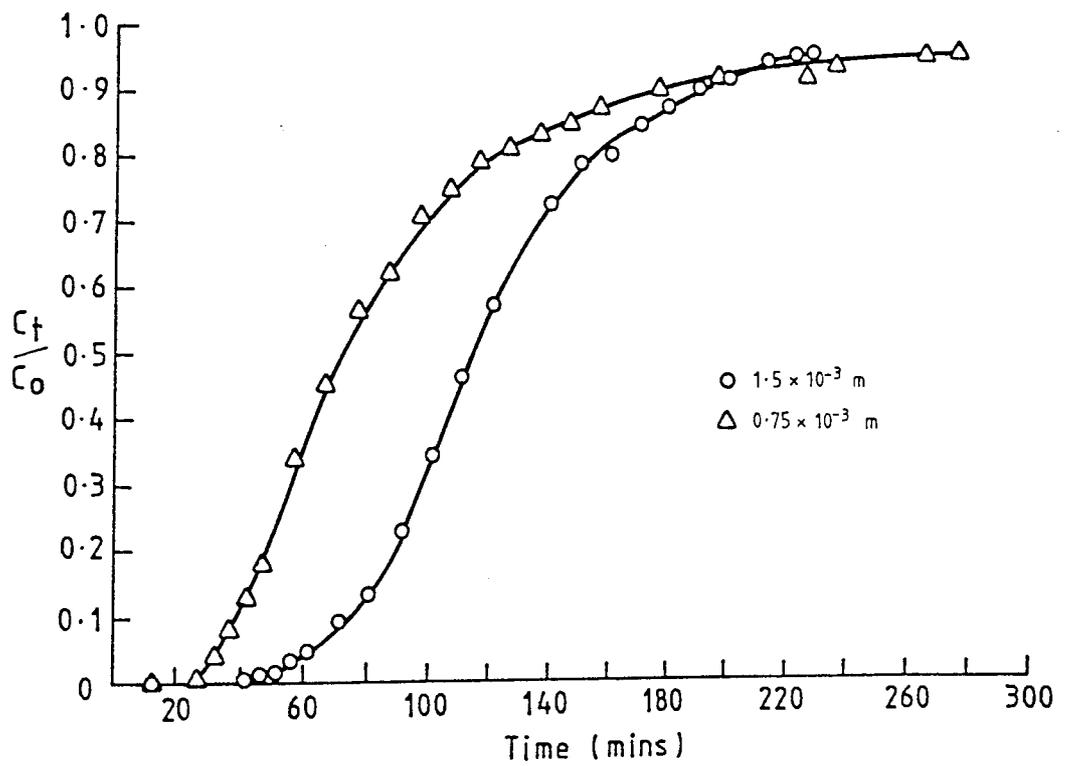
Figure 9.33 Effect of particle size (average diameter  $d_p$ ) on breakthrough curve of n-ecosane
