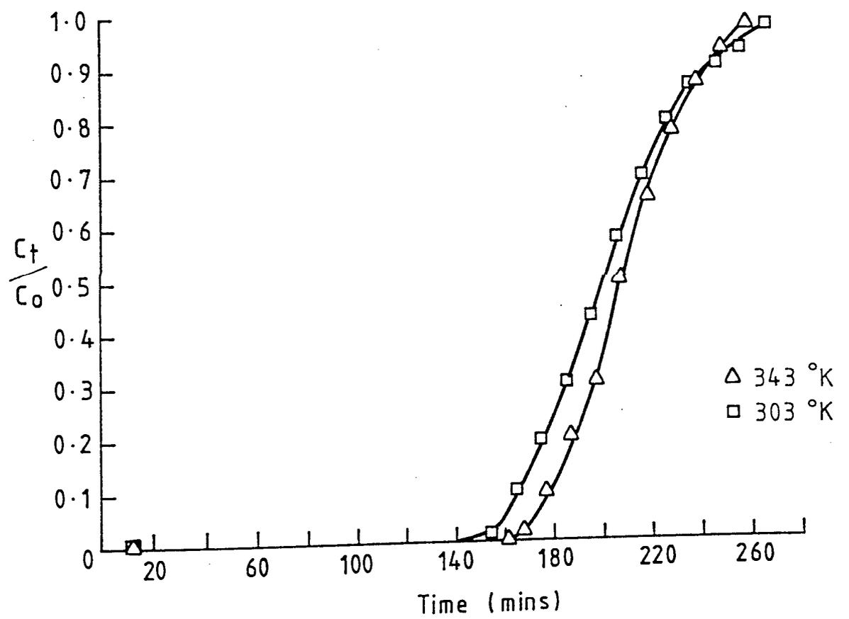
Figure 9.21 Effect of temperature on breakthrough curve of n-hexadecane
