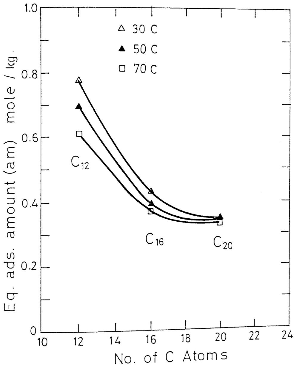
Figure 9.4: Plot of max. value adsorbed vs. n-paraffin carbon atoms.
