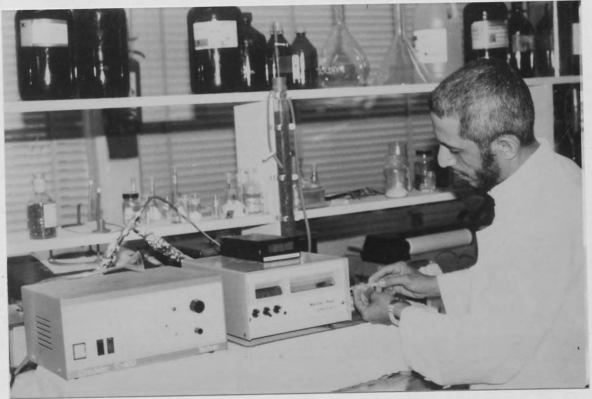
Figure 7.11 Injection of sample into the density meter
