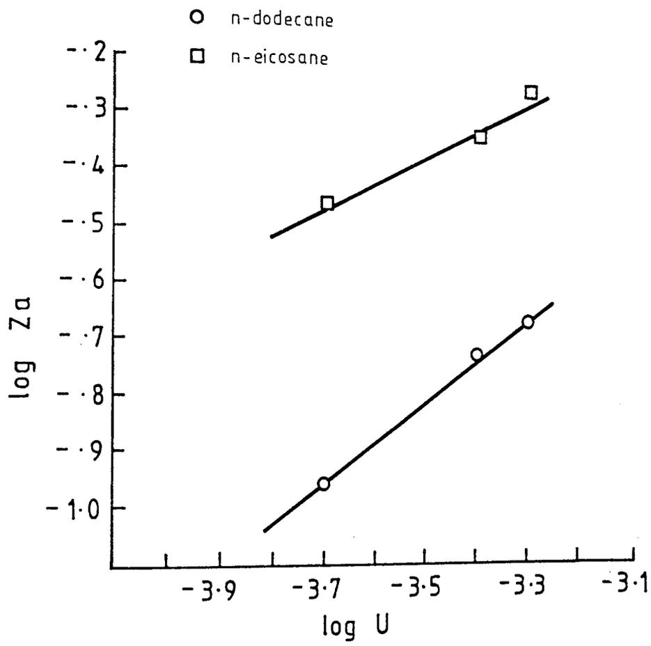
Figure 9.34 Effect of superficial velocity on adsorption zone height
