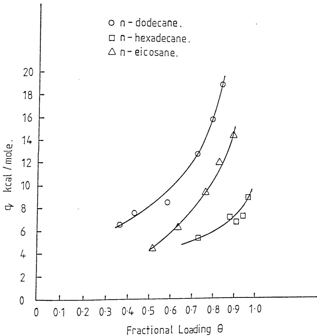
Figure 9.8 Variation of  $q_{150}$  with fractional loading for sorption of n-paraffins on 5A molecular sieves at 323°K
