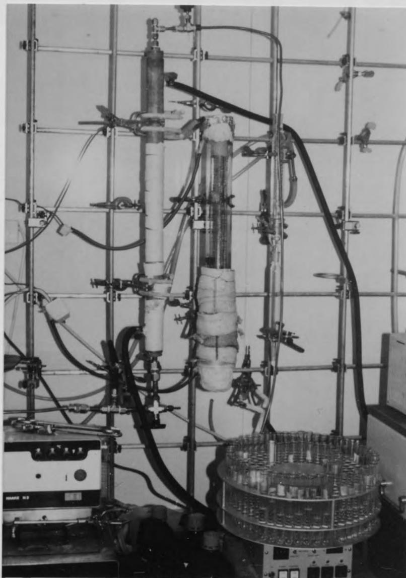
Figure 7.6 Adsorption and activation columns
