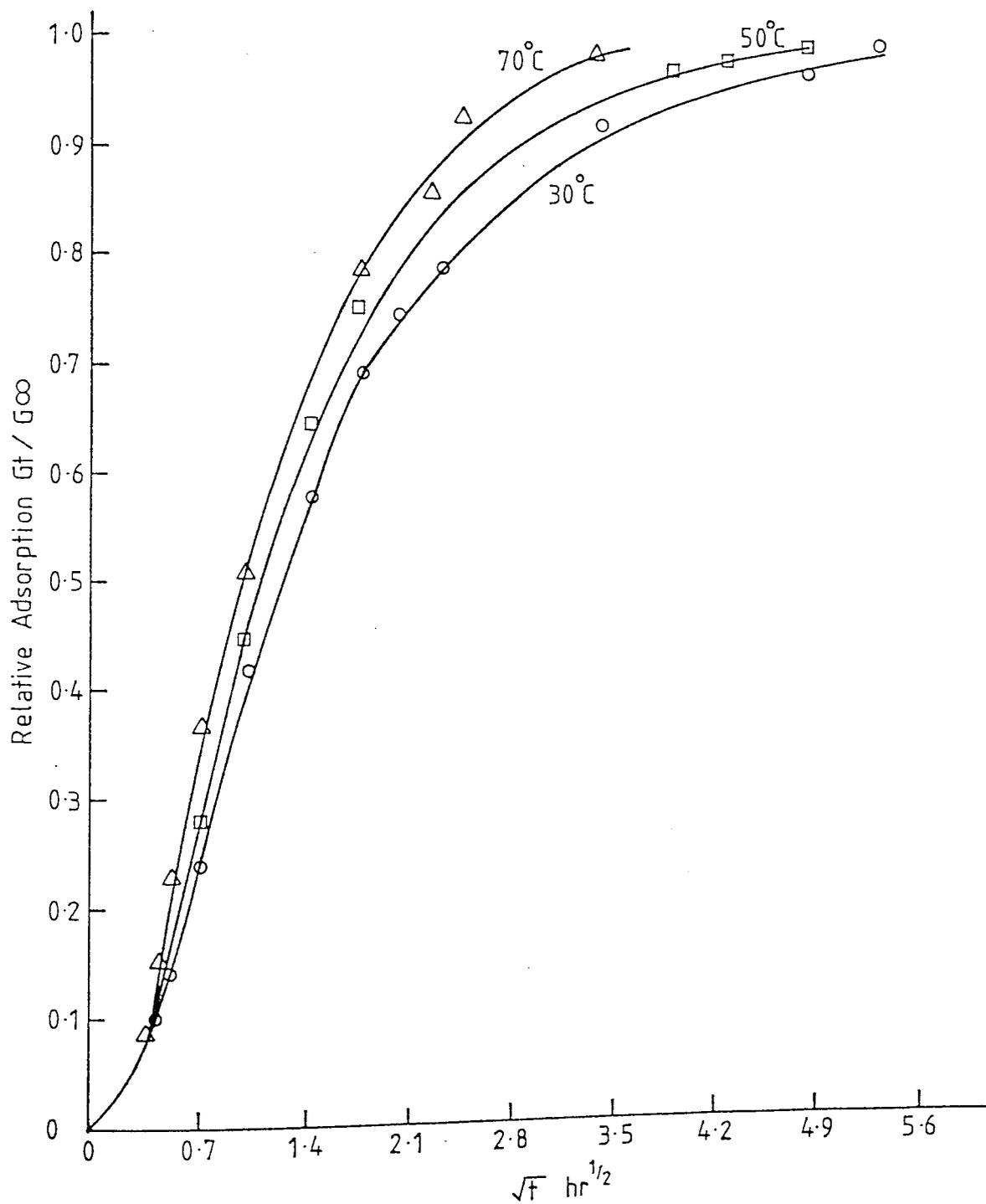
Figure 9.11 Kinetics of adsorption of n-eicosane from isooctane solution at various temperatures
