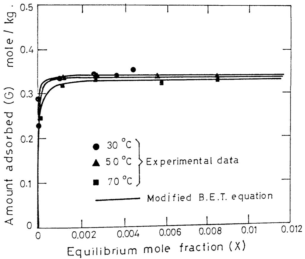
Figure 9-3: Adsorption isotherms of n - eicosane
