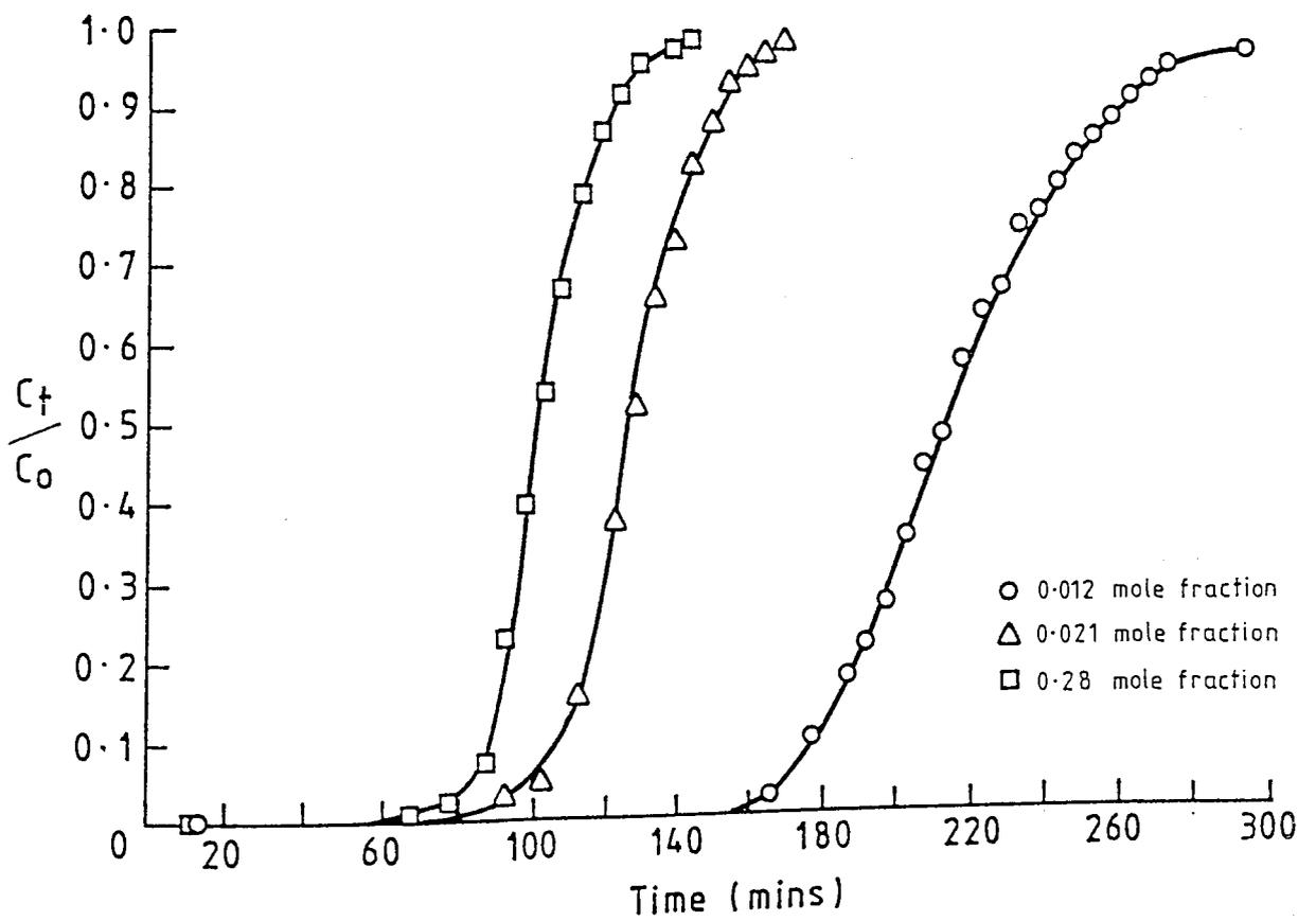
Figure 9.26 Effect of feed concentration on breakthrough curve of n-dodecane
