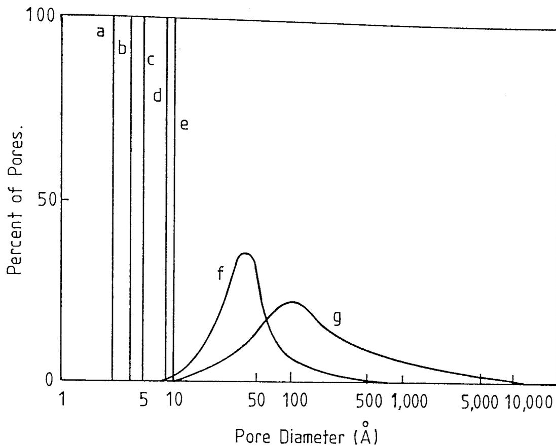
Figure 3.1 Typical pore size distribution, illustrating that molecular sieves have precise pore diameters.
