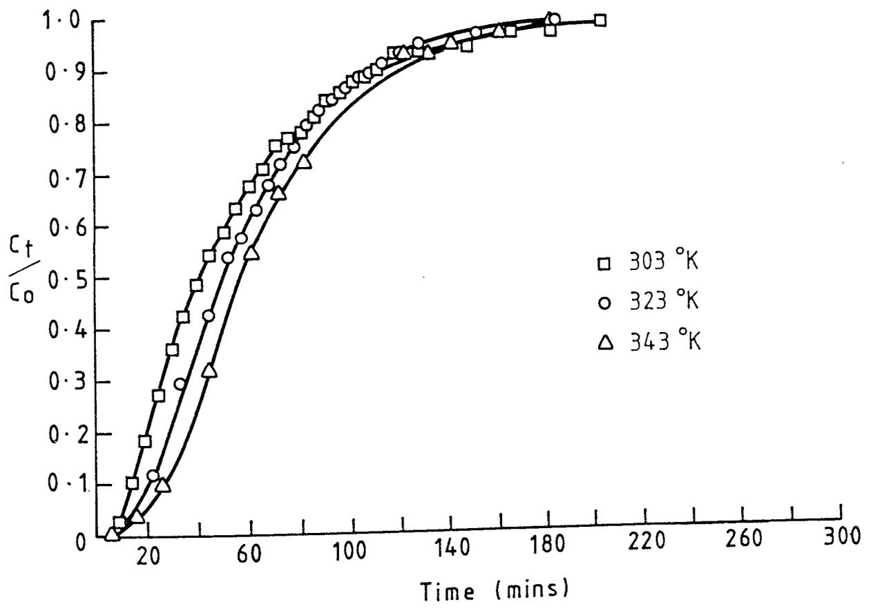
Figure 9.22 Effect of temperature on breakthrough curve of n-eicosane
