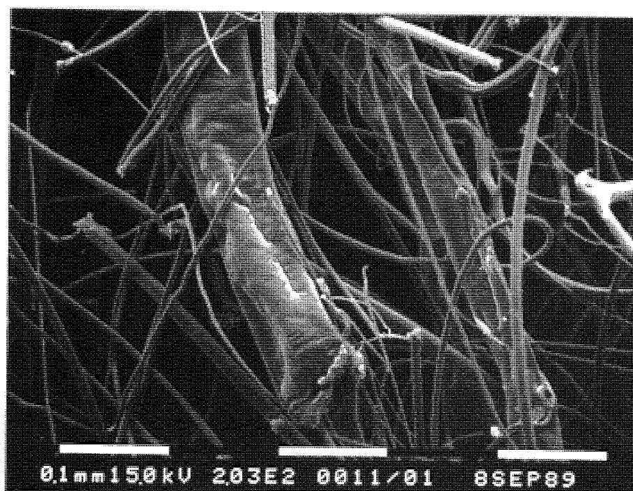
Plate 5.2: NOM 238 cell attachment on dichloromethane extracted PHB "wool".
