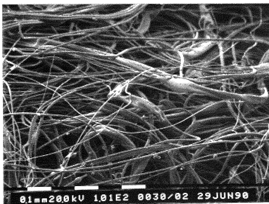
Plate 5.14: L929 cell attachment on 1% \text{H}_2\text{SO}_4 treated dichloromethane extracted PHB NWM.
