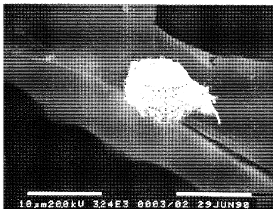
Plate 5.4: NOM 238 Cell attachment on 1% \text{H}_2\text{SO}_4 treated dichloromethane extracted PHB "wool".
