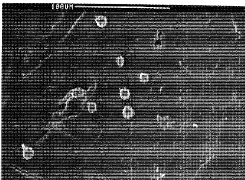
Plate 4.6: L929 cell attachment on 12% HV/30% Amylose copolymer.
