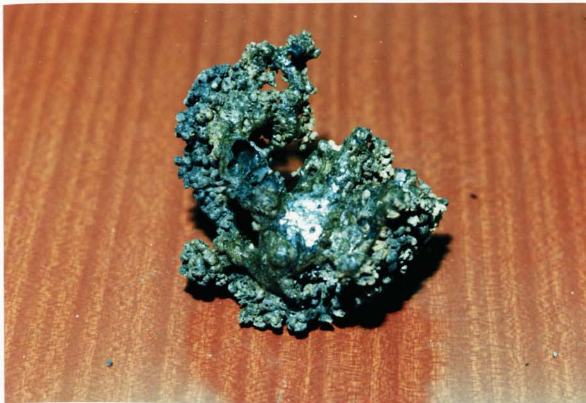
Figure 7.20 Clinker of Sewage Sludge Removed from Reactor After Test 10
