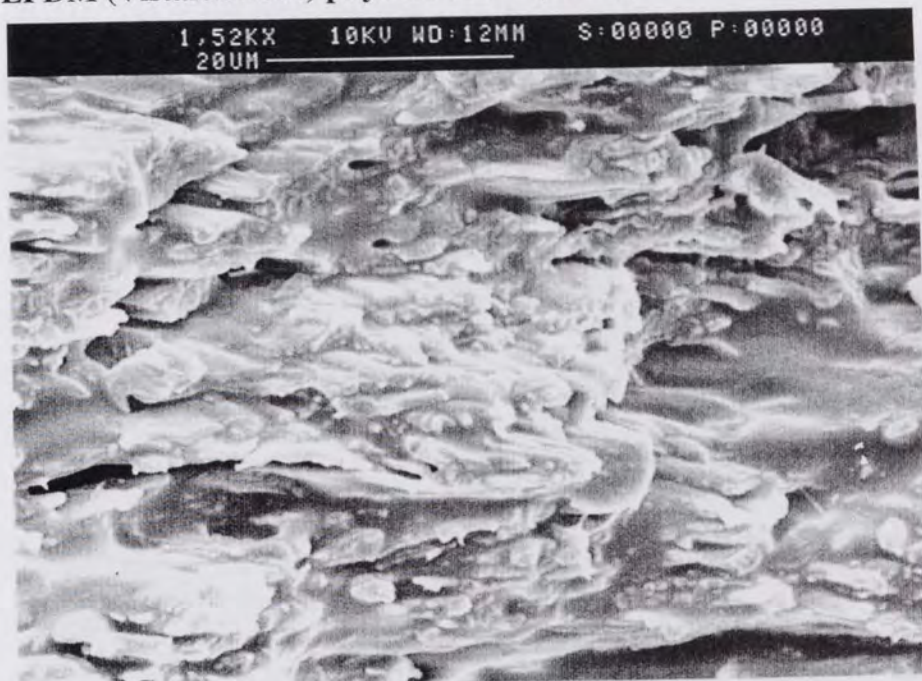
Figure 5.5 View of fracture surface from tensile test using scanning electron microscopy to show internal structure of 70/30 PS (Huntsman 311) / EPDM (Vistalon 2504) physical blend (1KA7).
