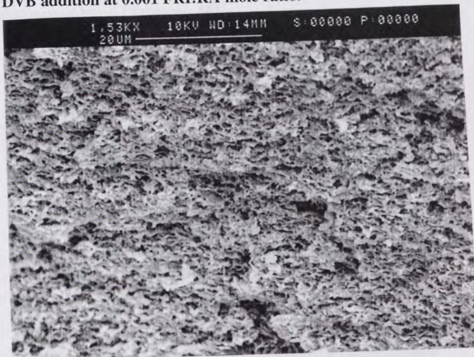
Figure 5.9 View of fracture surface from tensile test using scanning electron microscopy to show internal structure of 70/30 PS (Huntsman 311) / EPDM (Vistalon 2504) blend (5KA8) reactively processed with 5% DVB addition at 0.001 FRI:RA mole ratio.
