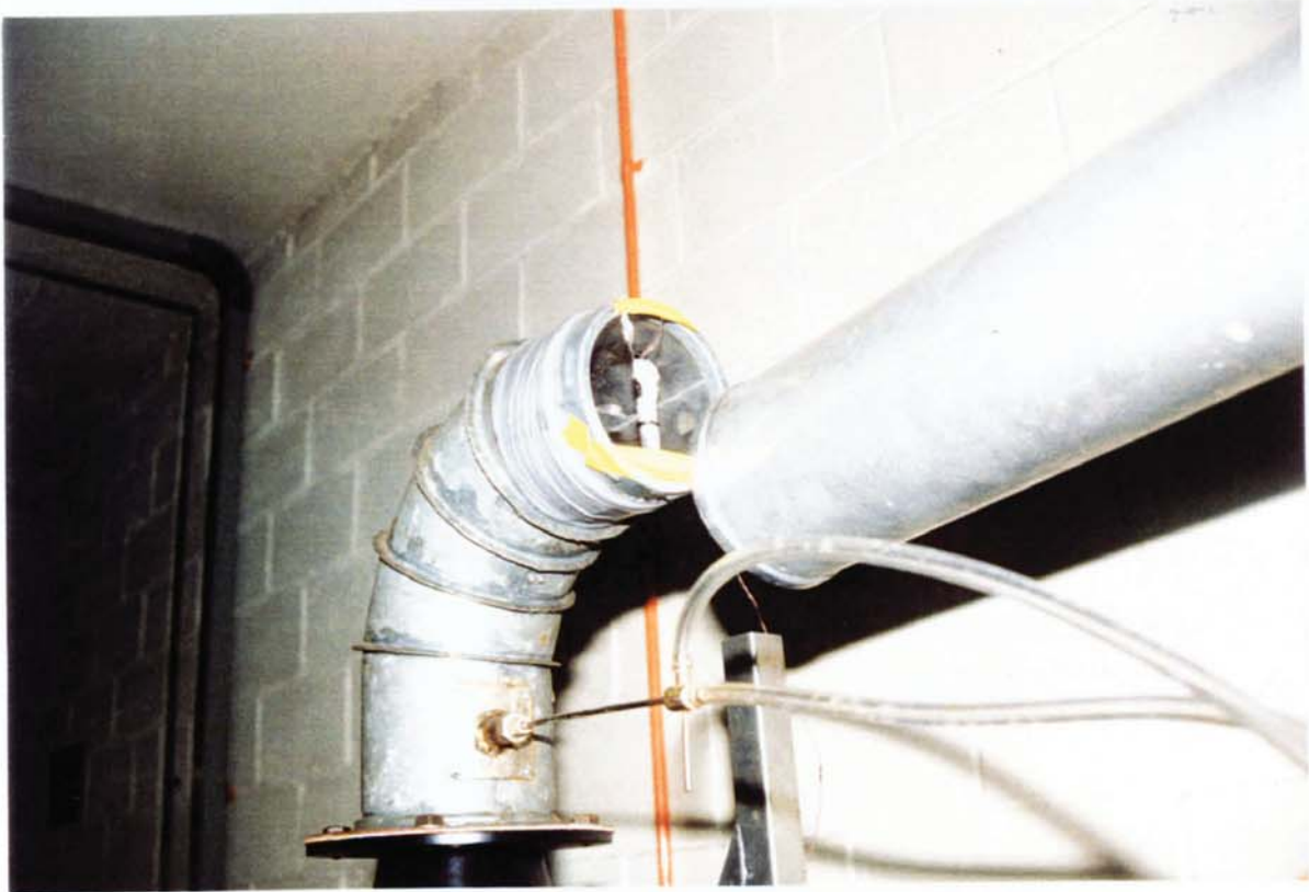
Plate 5.8 The Wet bulb Thermometer Assembly.
