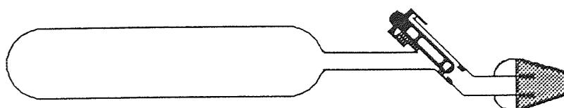
Catalyst solutions were prepared under argon using the Schlenk technique (see section 2.2) and stored in flasks of the type shown in figure 2.5. The solution was made up by injecting the initiator (or cocatalyst) into the large bulb of the catalyst flask into which excess solvent was distilled.
