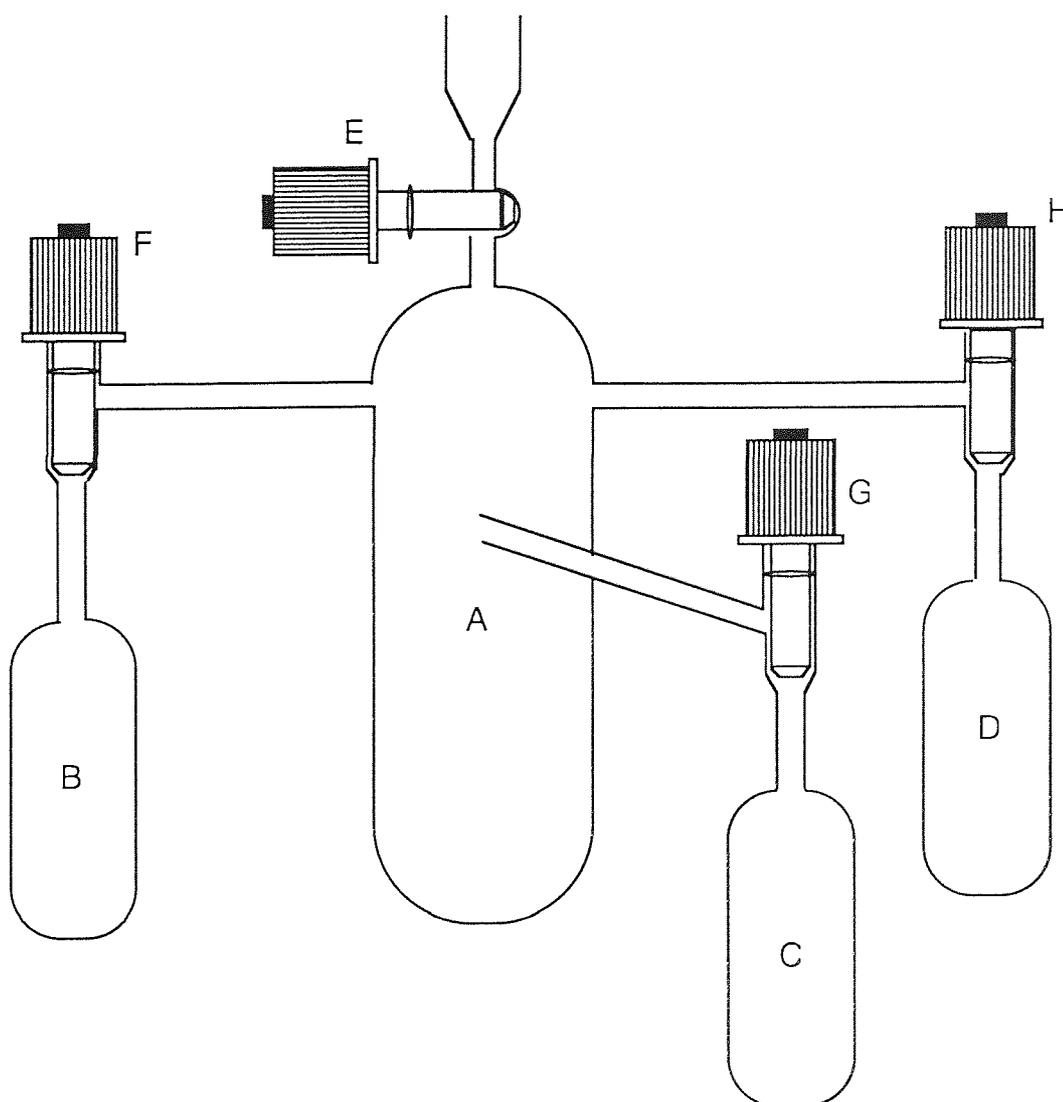
Typically, the monomer, e.g methyl methacrylate, was distilled into bulb B along with some solvent. The cocatalyst solution lithium chloride or aluminium alkyl, was then injected using the Schlenk technique into bulb C via tap G and a portion of the solvent required was also distilled into the bulb. The initiator, butyllithium, was injected via tap H
