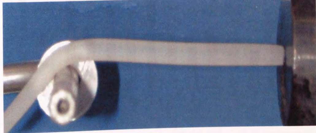
Figure 5.2 Effect of processing of stabilised polymers on the appearance of the extruded laces (4mm die) of m-LLDPE and z-LLDPE polymers extruded under the same conditions (using formulation s-4, see table 5.1). Clear melt fracture is shown in the case of the metallocene polymer.
