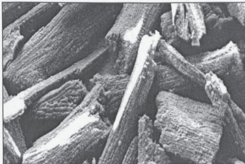
Figure 5.23: Surface structure of washed feedstock of size 355-500 \mu m
