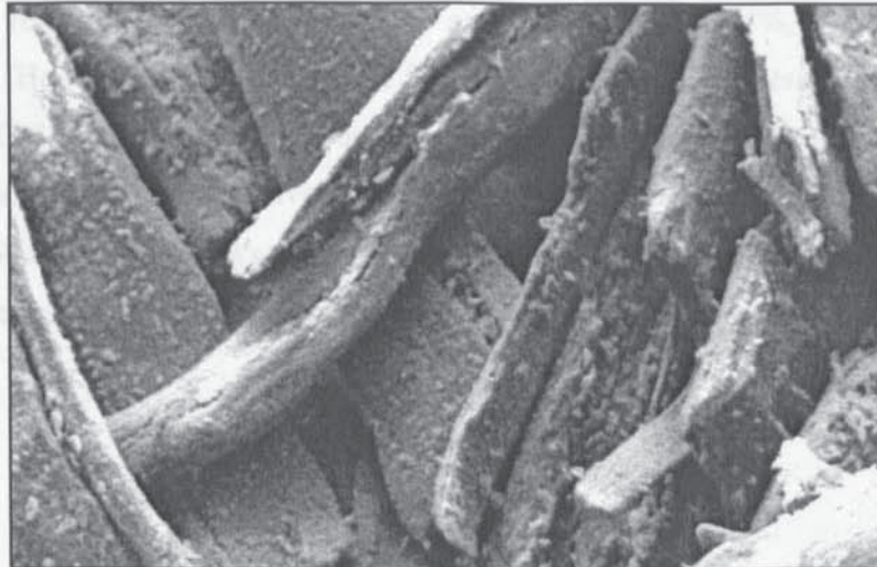
Figure 5.22: Surface structure of unwashed feedstock of size 355-500 \mu m
