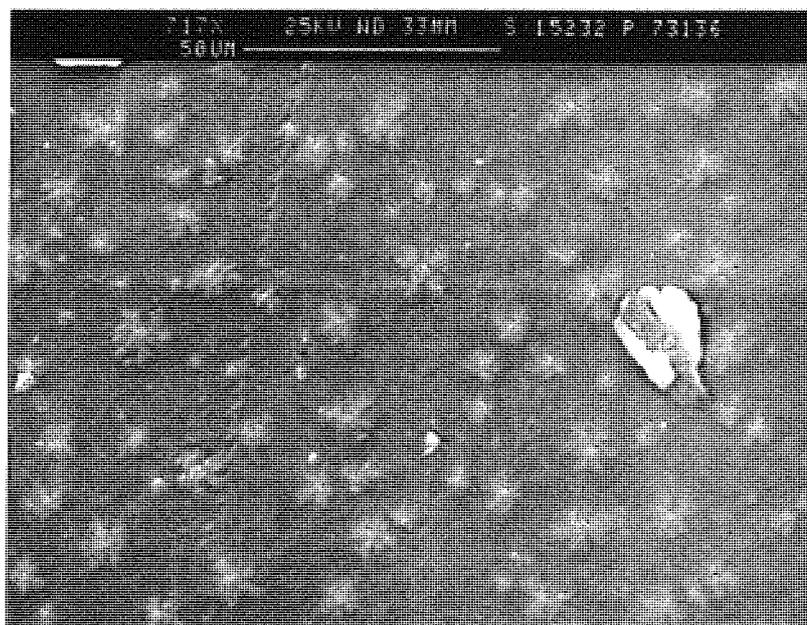
Figure 8.15 SEM micrograph of the surface of a HEMA hydrogel modified with 20 weight% of PEG1000MA
