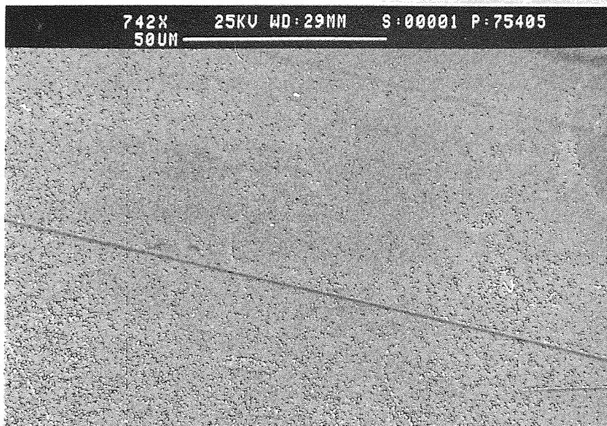
**Figure 8.17 SEM micrograph of the surface of a HEMA hydrogel modified with 20 weight% of PEG200MA**
