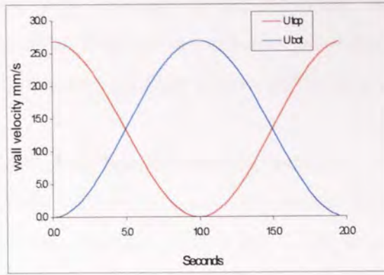
Figure 2.3a. Smooth curve representing the wall movements of the two dimensional cavity system, from equations 2.1 and 2.2
