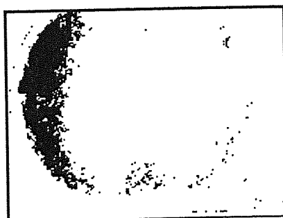
Figure 7.2c Binary Dye Images for the STR-2 Tray at Weir Loading of 50 \text{ cm}^3 \text{ cm}^{-1} \text{ s}^{-1} and Air Velocity of 0.8 \text{ m s}^{-1}
