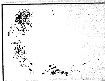
Figure 7.2a Binary Dye Images for the UMD Tray at Weir Loading of 50 \text{ cm}^3 \text{ cm}^{-1} \text{ s}^{-1} and Air Velocity of 0.8 \text{ m s}^{-1}
