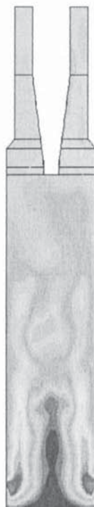
Figure 91 Pyrolysis reactor with two feed points, plot shows concentration of organic vapours (L)
