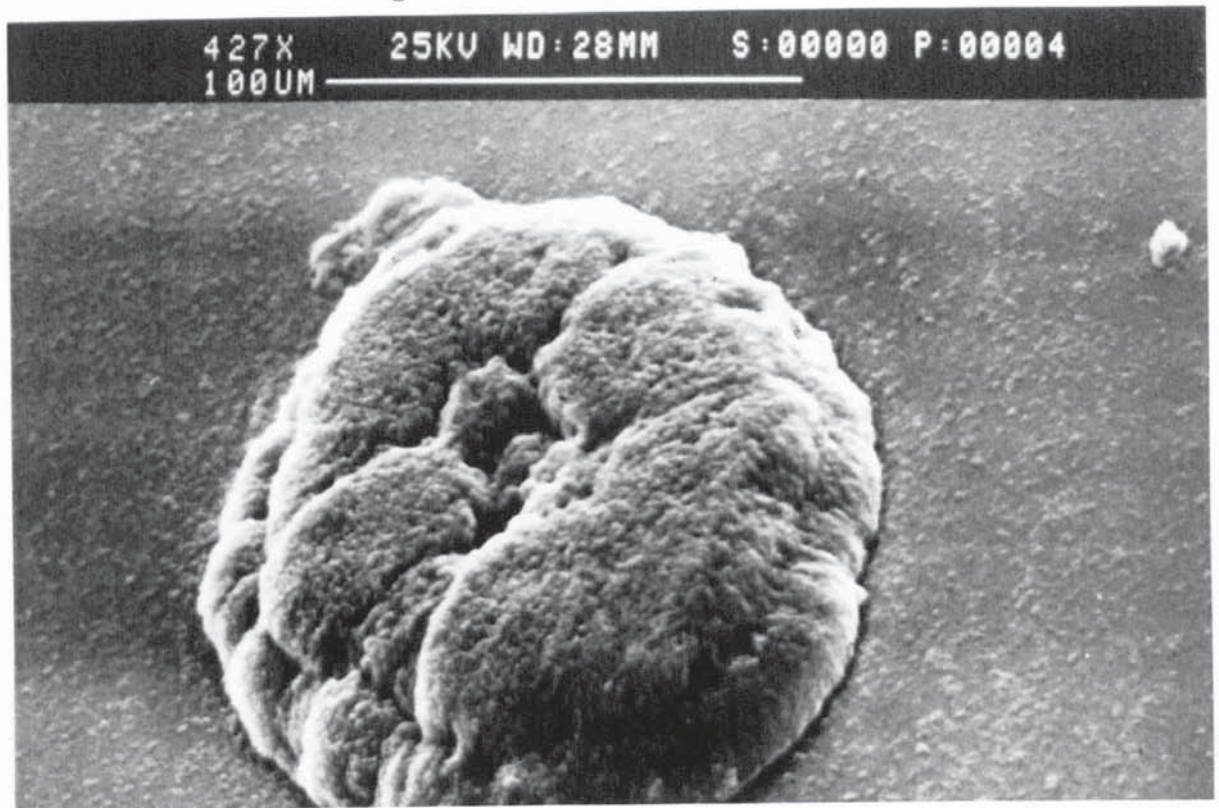
Figure 3.20 - SEM of a lens calculus from a high water content lens worn for six months
