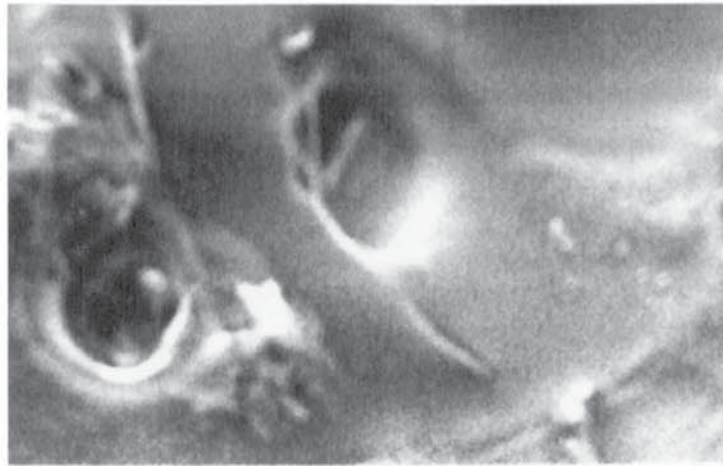
Figure 5.12 S.E.M. image of a Zinc Oxide Strip control on 116 x 200 \mu\text{m} magnification at 25kV Zinc Oxide control.
