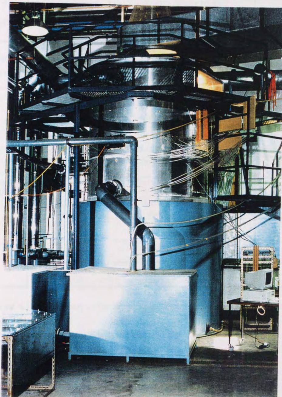
Fig. 4.2 Photograph of the air water simulator
