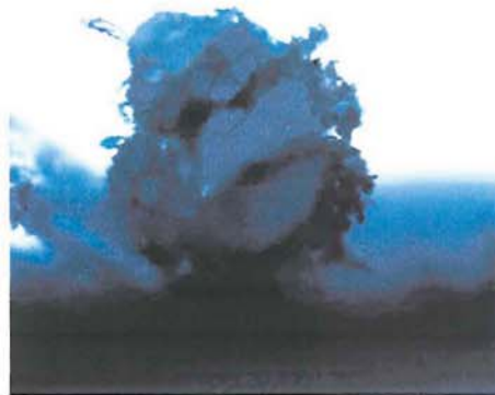
Figure 5-19: Fraying observed with the FMPengPOF over time after cleaving; image taken with \times 20 objective.
