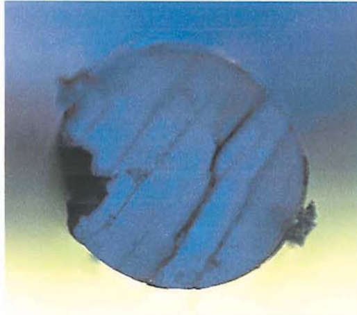
Figure 5-18: Cleaving FMPengPOF using liquid nitrogen and a razor blade; image captured with \times 20 objective.
