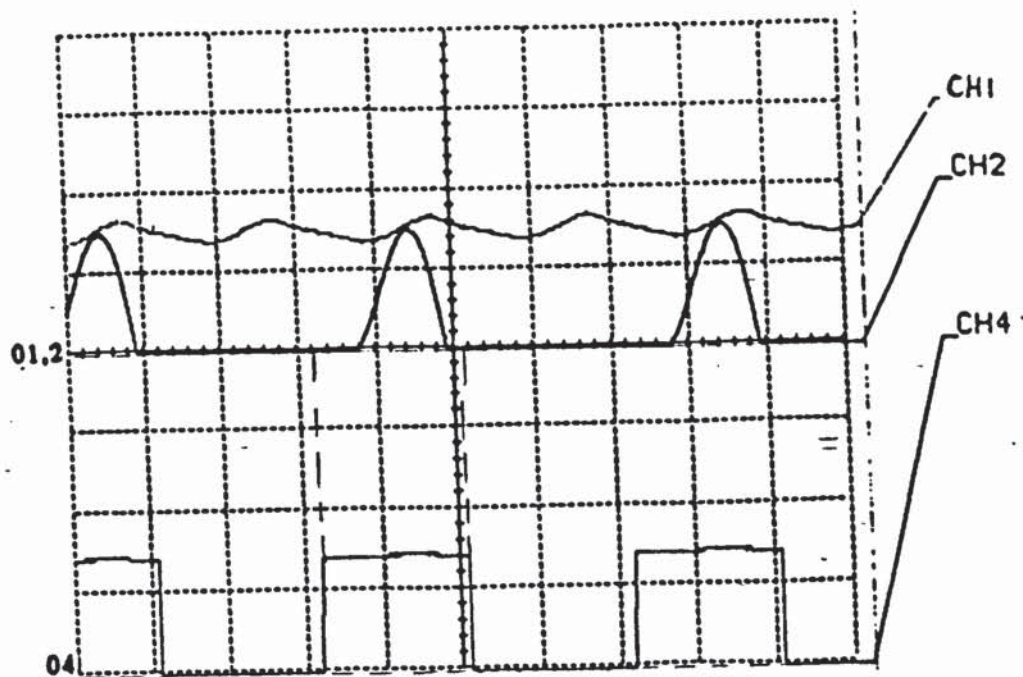
Figure (5-9) Steady-state condition when converter (A) operates as a rectifier (resistive load).
