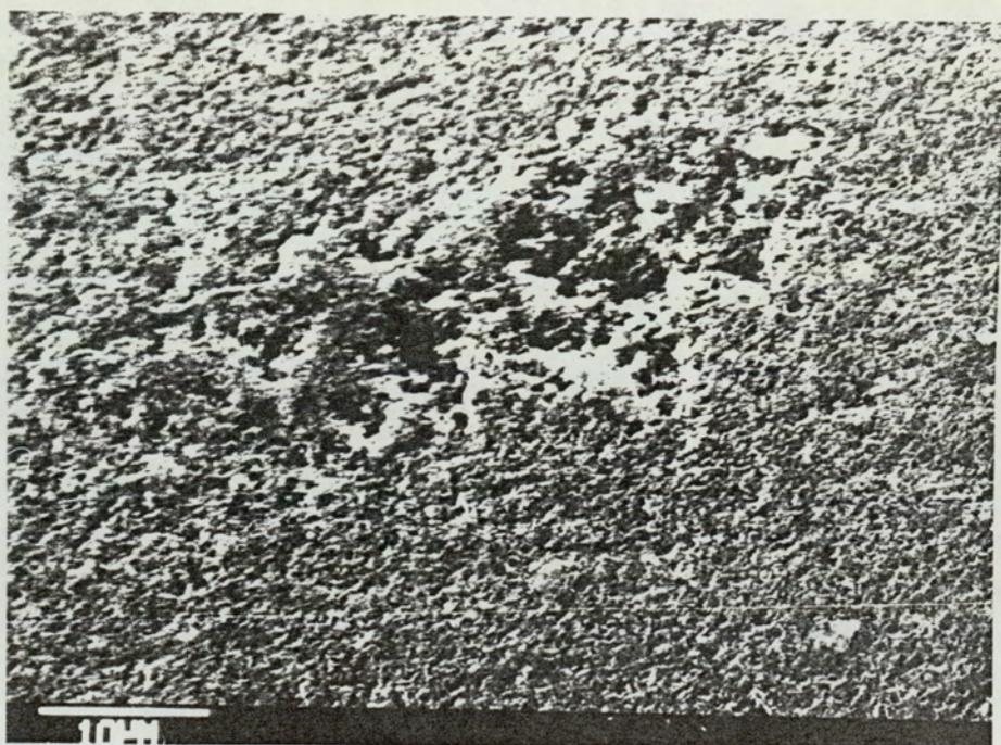
Figure 6.31 (a) Clear ploughing type plastic deformation on a sample tested on the simulation rigs.
