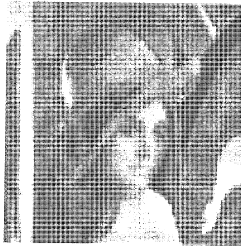
Fig. 2.12. Blockiness due to sub-sampling
