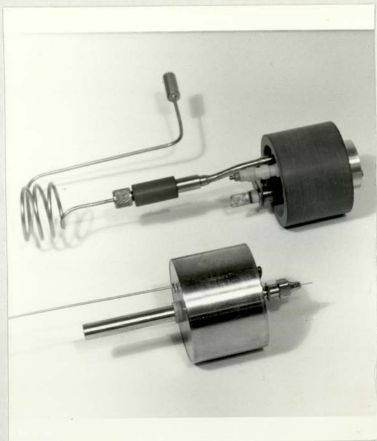
Fig.3.8 (a) Ion-Beam Module (b) Gas Sputtering Module
