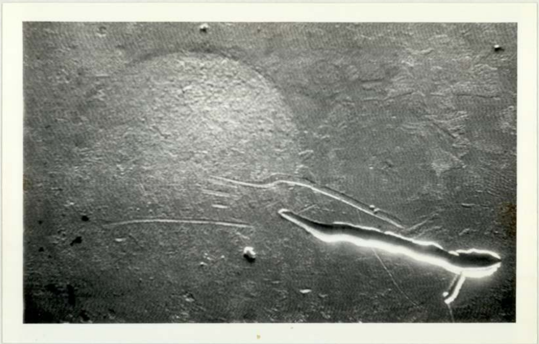
Fig.5.20 Marked Emission Site With Heavy Surface Damage Nearby
