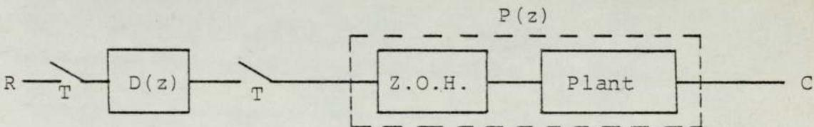
Fig. 2.1 System with series compensator  $D(z)$
