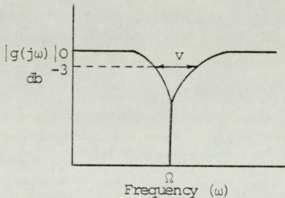
Fig. 4.4 Frequency response characteristics of the notch filter
