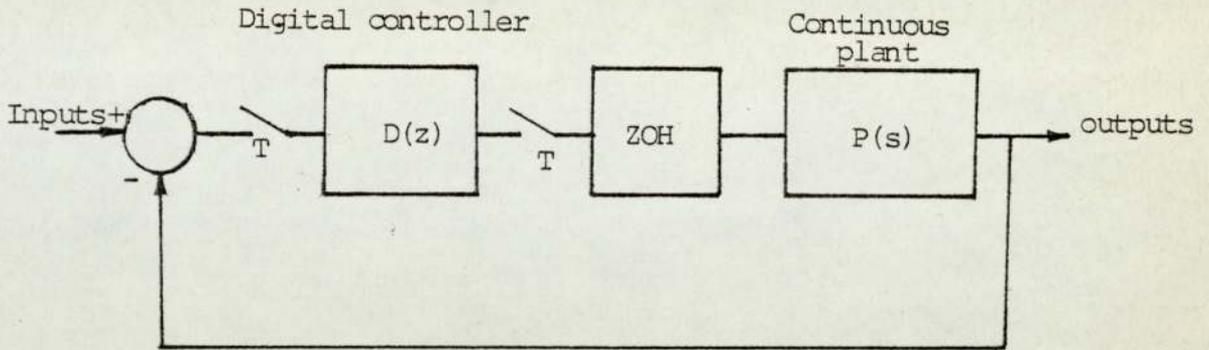
Fig. C.1 Digital control system for simulation
