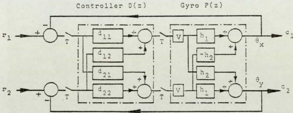
Fig. 1 Rebalance control system
