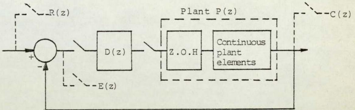
Fig. 3.1 System Configuration
