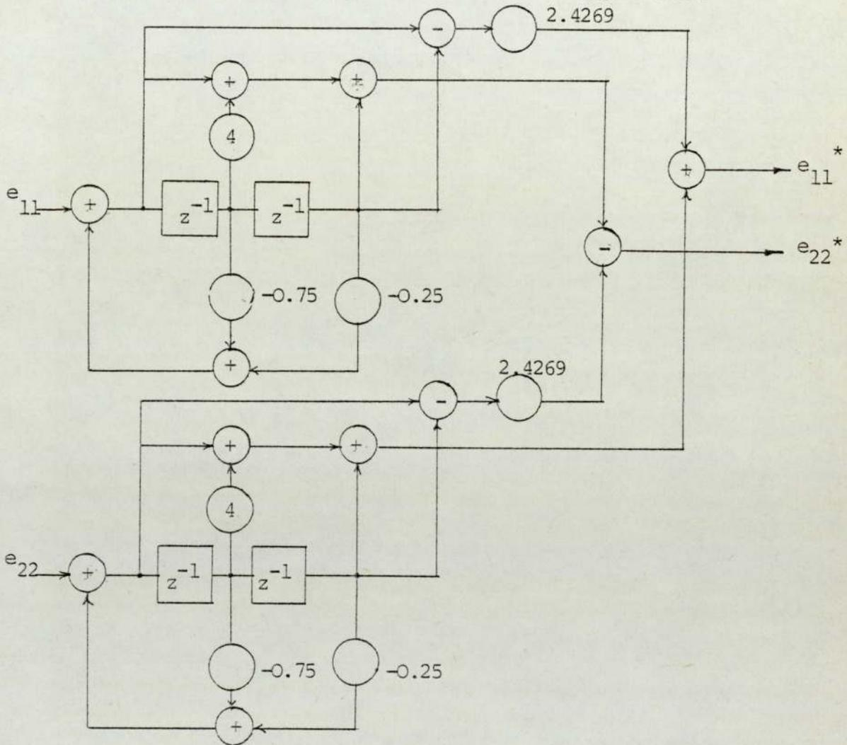
Fig. 5.1 Implementation of control algorithm for class I design
