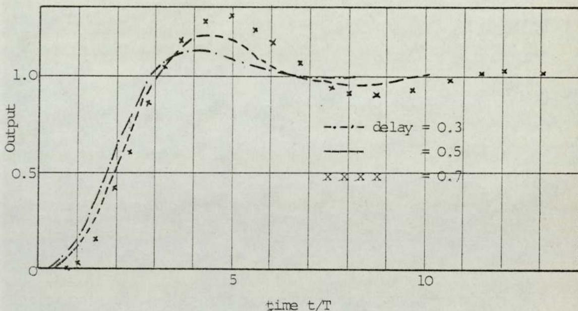
Fig. 4.5 Response with processing delay
