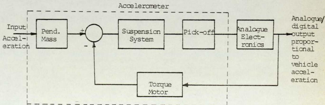
Fig. B.1 Block diagram of a pendulous accelerometer
