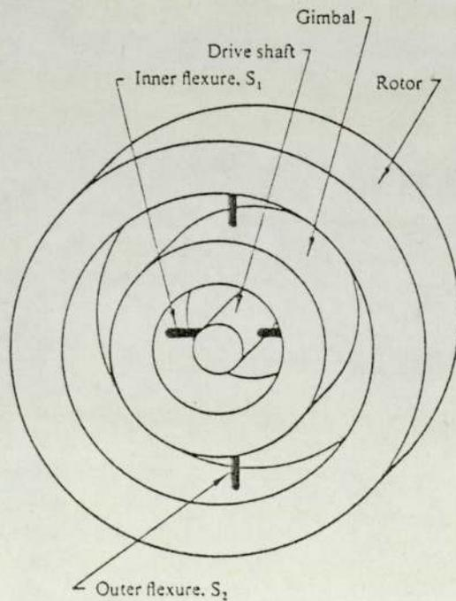
Fig. 1.1 Basic construction of a single-gimbal tuned gyro
