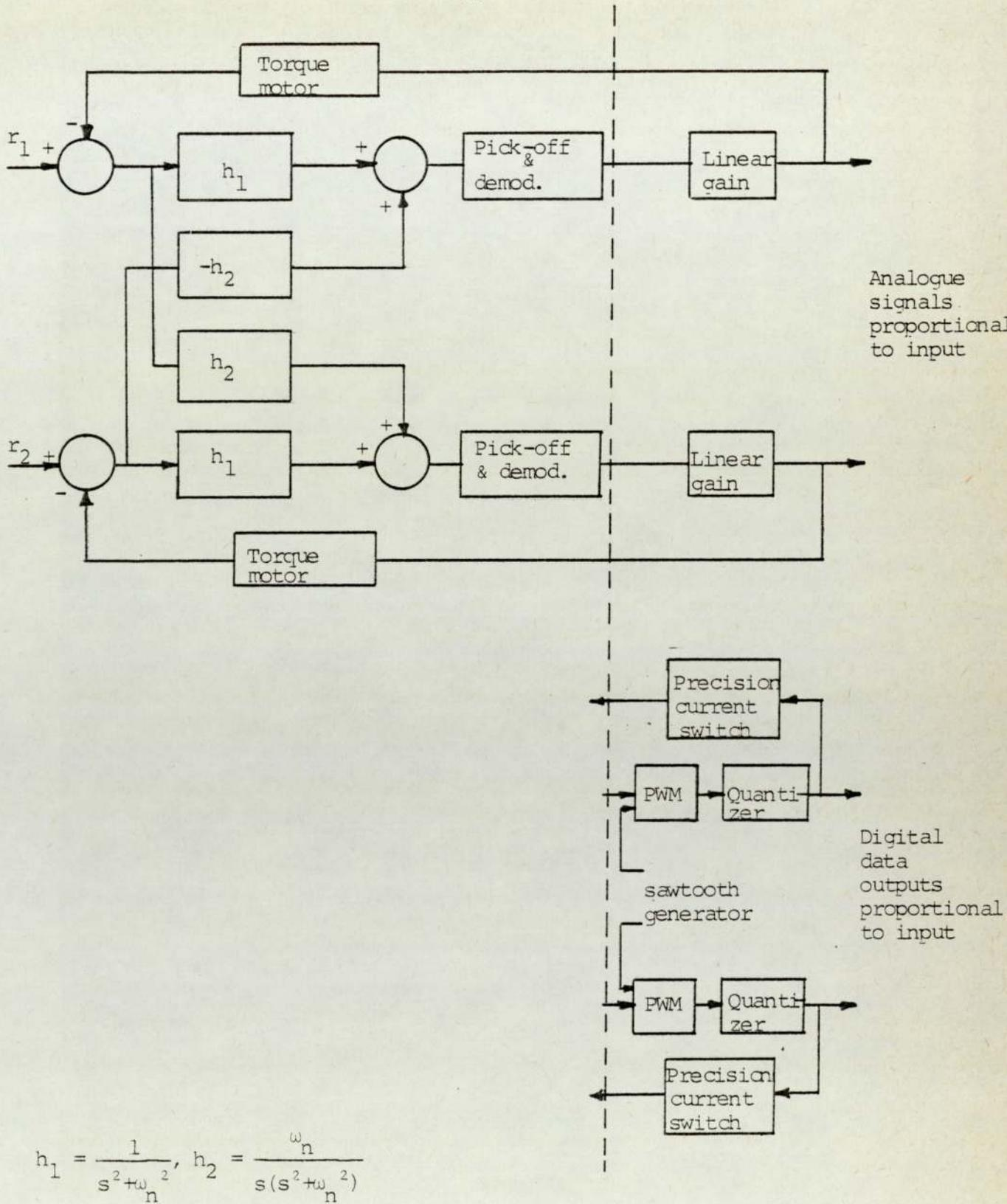
Fig. A.1 Analogue and BPWM rebalancing schemes
