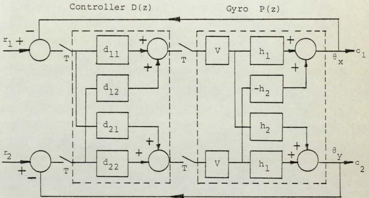
Fig. 1.2 Proposed direct digital control rebalance system
