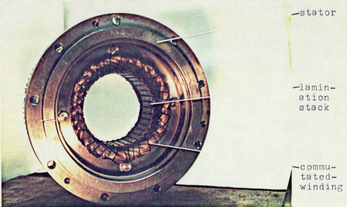
Photograph 2b Stator and commutated-winding (ODE) inside view
