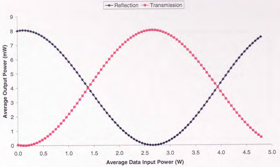
Figure 3.12: By varying the average power of the input data, the “clock” can be switched out of either of the two arms of the NOLM
