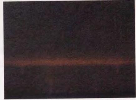
Figure 4.12 Photograph of the plasma - cathode sheath, 90 mT, 150 W, a) Ar + 50% O<sub>2</sub> b) Ar + 75% O<sub>2</sub>
