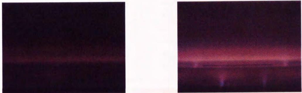
Figure 4.4 Photograph of the plasma - cathode sheath region; a) 90 mT, 5 W and b) 90 mT, 150 W (argon)
