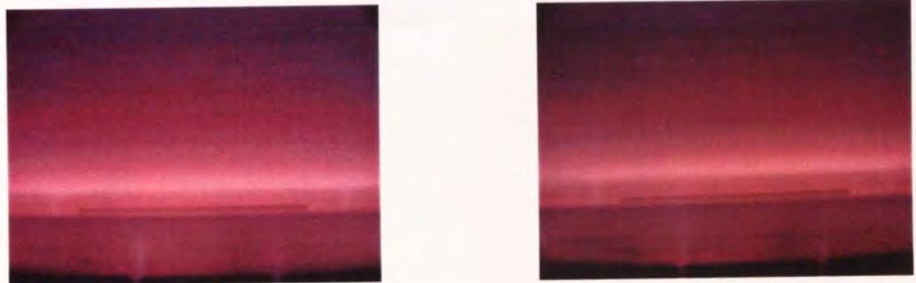
Figure 4.19 Photograph of the plasma-cathode sheath, 90 mT, 150 W, a) Ar + 50% H<sub>2</sub>, b) Ar + 75% H<sub>2</sub>
