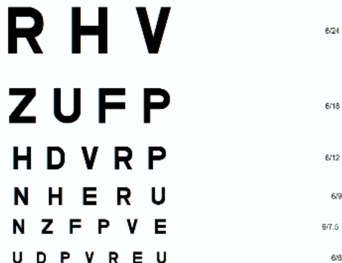
Figure 14. The Thomson XPert 3Di Snellen Chart: This chart is designed to present letters that subtend 5 minutes of arc vertically, scaled for different viewing distances. These letters are then presented at a consistent viewing distance, typically 6m (or 20 feet in USA and Canada). The chart is viewed at the distance required of the instrument, and the subject reads down until they are unable to correctly identify the letters. Scoring consists of a fraction, with the numerator consisting of the viewing distance while the denominator consists of the respective distance where the letters read subtend 5 minutes of arc. Missed or additional letters may be annotated, though due to the uneven scaling and number of letters on each line, results may vary between clinicians.
