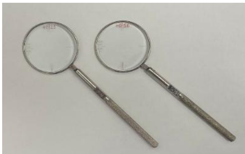
Figure 12. The Jackson Crossed Cylinder lens. The lens is a spherocylindrical combination lens where the resultant power is equal to the combination of two oppositely powered cylinders placed orthogonal to one another. The design of the JCC is such that the lens can be easily changed by rotation of the to alter the power presented to the subject, deriving power and axis through a series of forced choice presentations.
