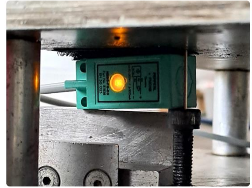
Figure 5. An inductive proximity sensor detects the pin placed in front of its detecting face.
