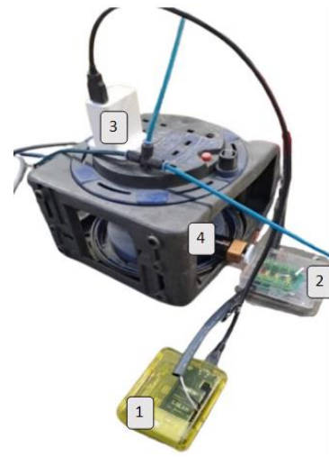
Figure 6. Hardware connections used on the machine for machine monitoring: 1) Microcontroller (NodeMCU), 2) Optocoupler Relay, 3) Power supply from the AC power socket outlet to the NodeMCU, 4) Power supply from the 9V battery to the proximity sensor.
