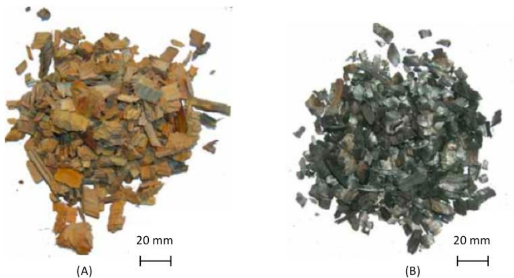
Figure 5.5: (A) raw wood chips, (B) charcoal after wood chip pyrolysis
