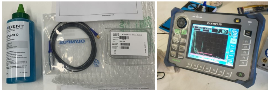
Figure 97 Ultrasonic transducer V203-RM and data collection equipment EPOCH 650.
