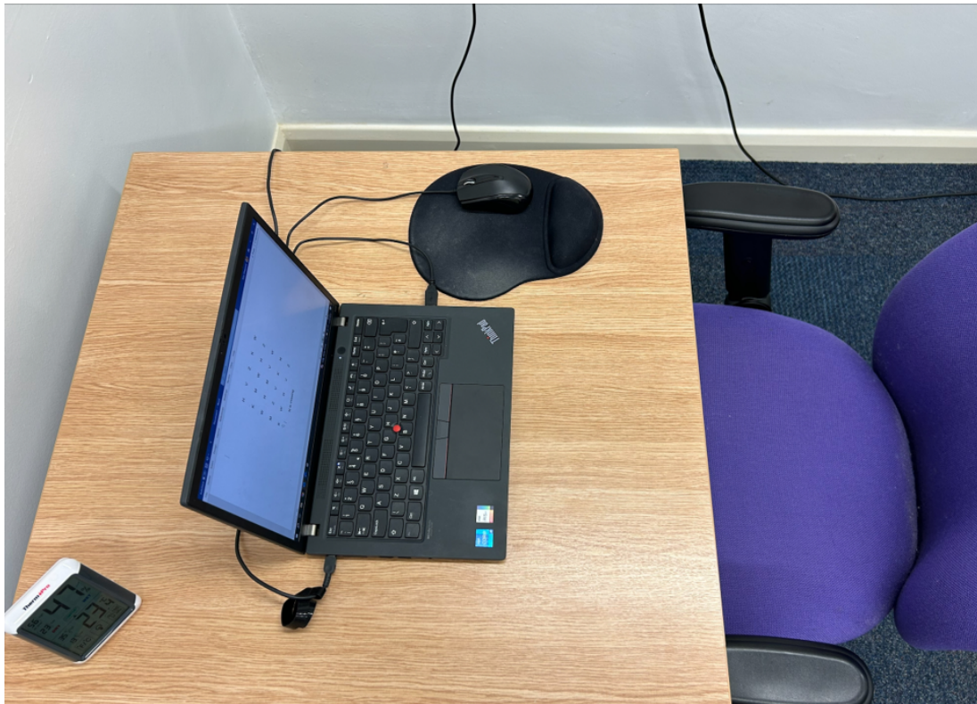
Figure 6.1. Photograph showing the real-world experiment setup. The laptop was viewed from a 50 cm working distance with the room lights on. Room temperature and humidity were monitored and recorded at each visit.
