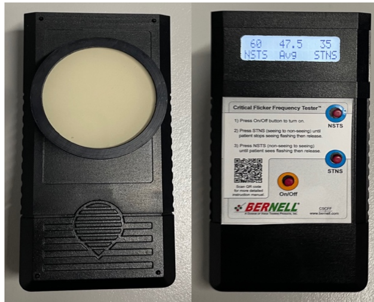
Figure 3.1. Front and back images of the Bernell pocket CFF tester (Bernell Corporation, Mishawaka, USA). On the display screen, 60 NSTS refers to 60 Hz non-seeing to seeing, 35 STNS refers to 35 Hz seeing to non-seeing and 47.5 Avg refers to the average CFF value which is 47.5 Hz.
