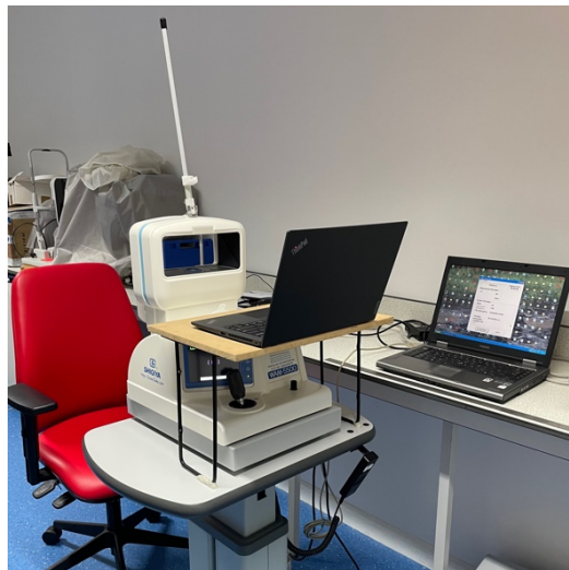
Figure 2.8. The set-up whilst measuring the dynamic refraction and pupil size with the Grand Seiko Auto Refractor / Keratometer WAM-5500 (Grand Seiko Co. Ltd., Hiroshima, Japan).
