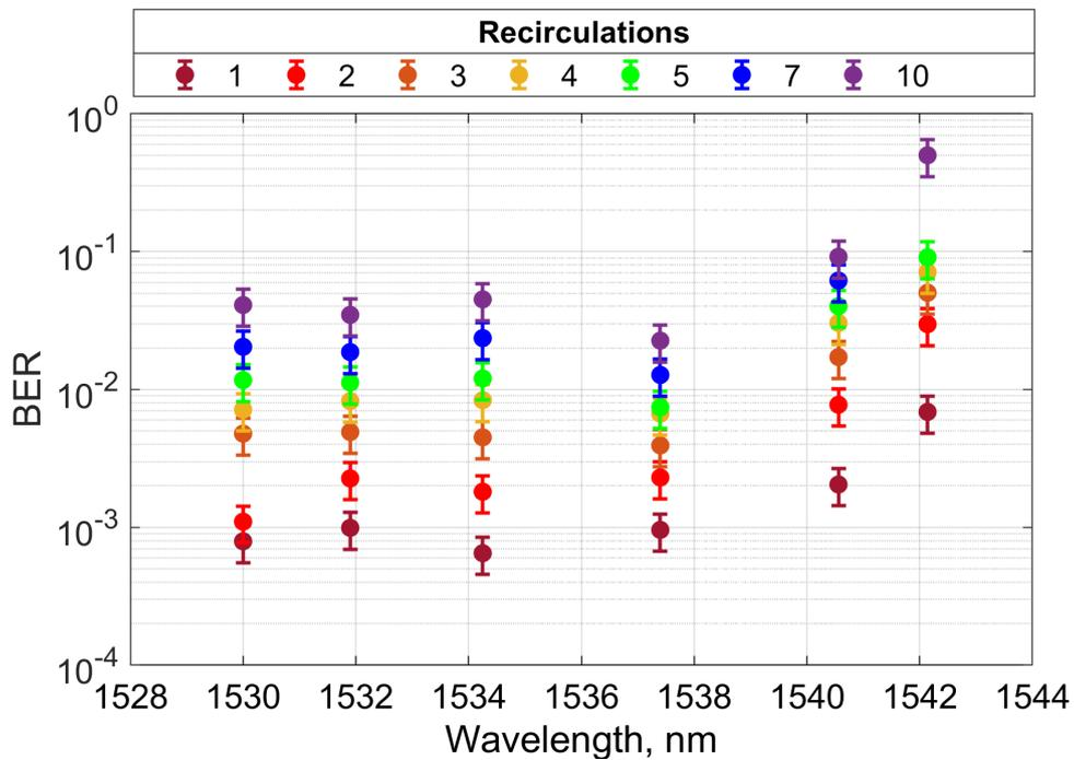
Figure 59. BER versus wavelength for number of recirculations.
