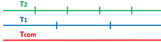
Figure 2.2: The schematic of commensurable periods with T_{com} being a common multiple for all others.
