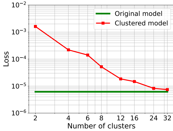
Figure 2.16: Loss function estimated on test data for the different numbers of clusters and loss of the baseline model (cited from [CP1]).
