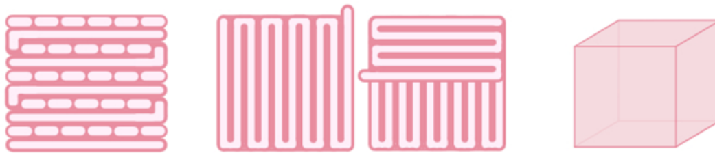
Figure 2. Example of additive layer manufacturing approach to 3D printing, enabling generation of macroscale structures via extrusion of a singular filament into a lattice structure (left to right; side view, birds eye view, final construct). Fusion of printed material enables production of a monolithic constructs.
