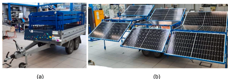
Fig. 14. Mobile solar power energy storage system showing (a) System folded (b) System unfolded.
