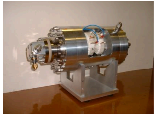
Fig 5. Photograph of the prototype linear compressor (Liang, 2014).
