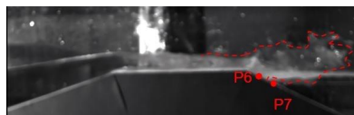
487 Fig. 14. Overtopping pattern of the overtopping jet flow just as it contacts the rear slope at position P6 488 during the extreme wave overtopping process.
