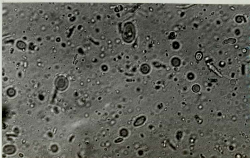
PLATE 4.10. BATCH 2 - GOOD EMULSION 500 x MAGNIFICATION
