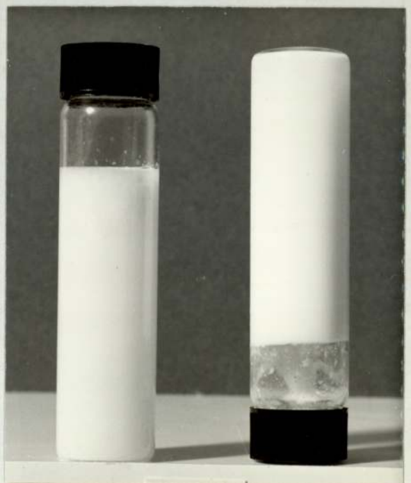
A - PLATE 4.8. BAD WAX EMULSION - B (ACCELERATED STORAGE)
