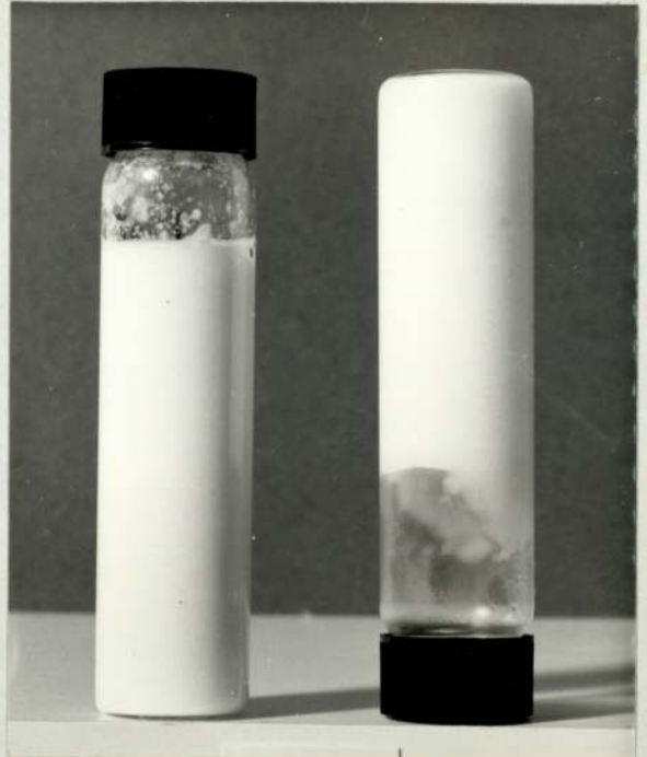
A - PLATE 4.6. BAD PRODUCT - B (ACCELERATED STORAGE)
