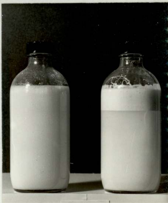
A - PLATE 4.4. - BAD EMULSION - B (AMBIENT STORAGE)
