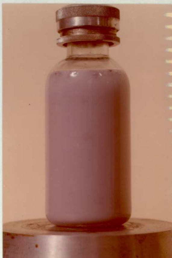
PLATE 6.17. Malformed Pressure Emulsion
