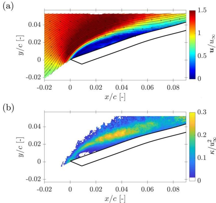
**Figure 10.** (a) Streamlines and contours of nondimensional flow velocity, and (b) contours of nondimensional turbulent kinetic energy (plotted for  $\kappa > 10^{-2}u_\infty$ ) for the leading edge of the 2D circular arc at  $\alpha = 25^\circ$  and  $Re = 53\,530$ .
