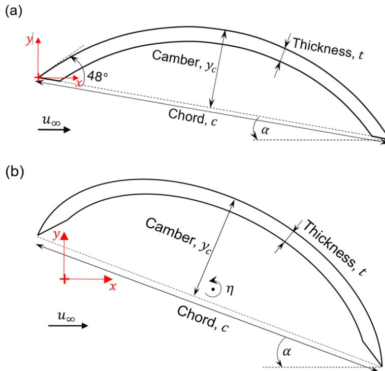
**Figure 1.** (a) 2D circular arc and (b) midspan section through the 3D sail, where  $\alpha$  is the angle of attack, and  $\eta$  is the rotation angle of the sail from its intended operating angle (Braun et al., 2016).
