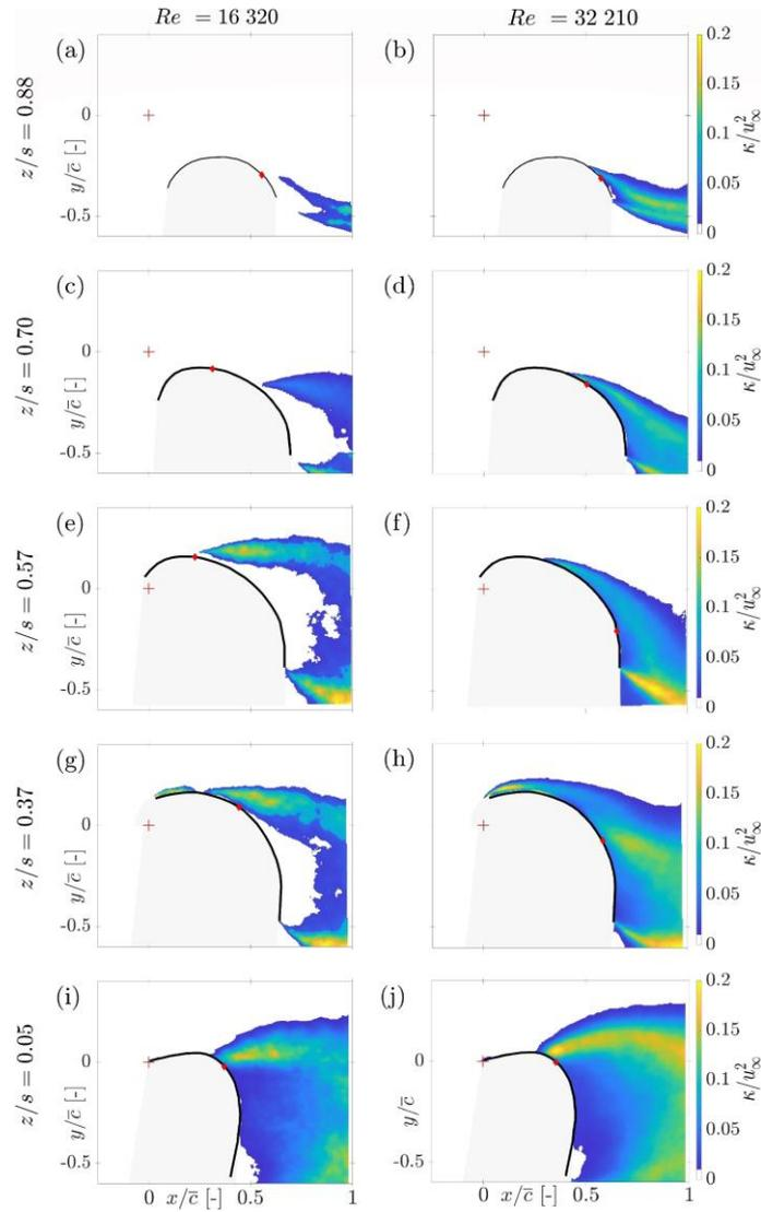
**Figure 12.** Contours of nondimensional turbulent kinetic energy (plotted for  $\kappa > 10^{-2}u_\infty$ ) for the 3D at  $\eta = 0^\circ$  for  $Re = 16\,320$  (left) and  $Re = 32\,210$  (right). Red diamond denotes the separation point.
