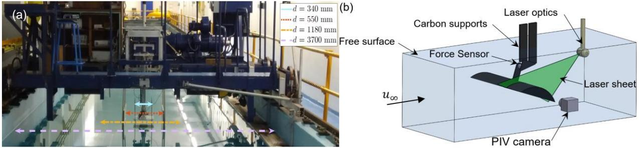
**Figure 2.** (a) 2D circular arc in the towing tank with sidewall locations, and (b) schematics of the PIV setup in the water tunnel.
