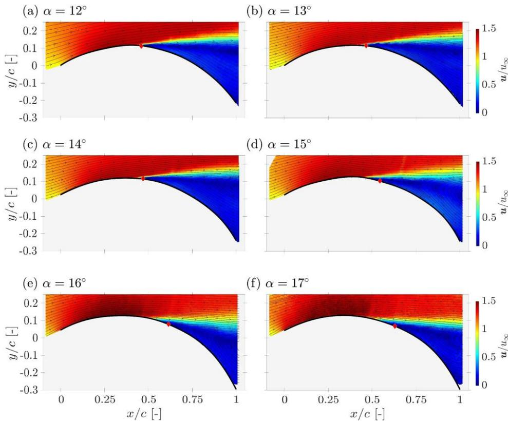
**Figure 7.** Streamlines and contours of nondimensional flow velocity for the 2D circular arc at  $Re = 68\,200$  for angles of attack of (a)  $12^\circ$ , (b)  $13^\circ$ , (c)  $14^\circ$ , (d)  $15^\circ$ , (e)  $16^\circ$  and (f)  $17^\circ$ . Red diamond denotes the separation point.
