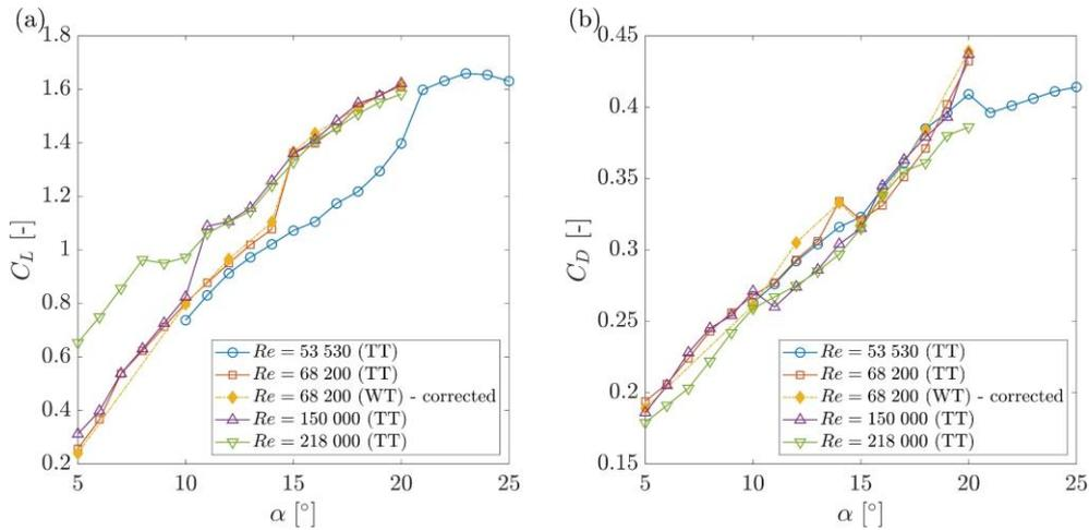
**Figure 4.** (a) Lift and (b) drag coefficients for the 2D circular arc at  $53\,530 \leq Re \leq 218\,000$ .
