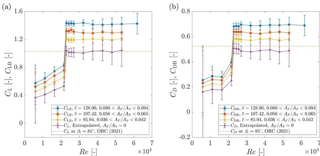
**Figure 6.** (a) Lift and (b) drag crisis versus for the 3D sail at  $\eta = 0^\circ$ .
