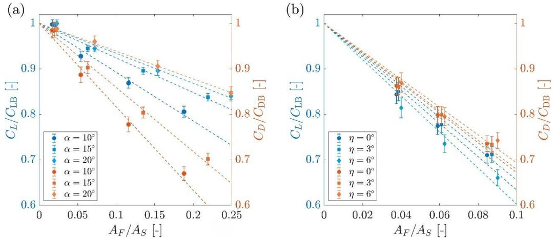
**Figure 3.** Effect of blockage ratio  $A_F/A_S$  for (a) the 2D circular arc and (b) the 3D sail.
