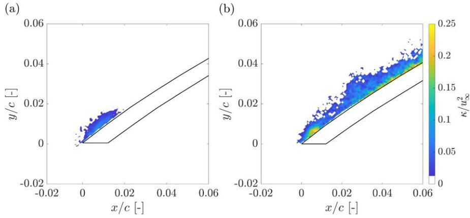
**Figure 9.** Contours of nondimensional turbulent kinetic energy (plotted for  $\kappa > 10^{-2}u_\infty$ ) for the leading edge of the 2D circular arc at  $Re = 68\,200$  for (a)  $\alpha = 13^\circ$  and (b)  $\alpha = 16^\circ$ .
