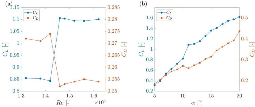
**Figure 5.** Force crisis for the 2D circular arc versus (a)  $Re$  at  $\alpha = 11^\circ$ , and (b)  $\alpha$  at  $Re = 68\,200$ .
