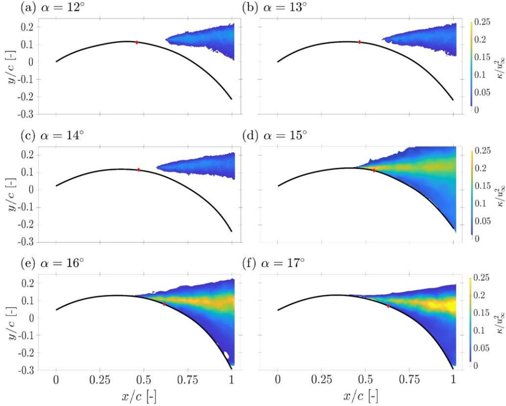
**Figure 8.** Contours of nondimensional turbulent kinetic energy (plotted for  $\kappa > 10^{-2}u_\infty$ ) for the 2D circular arc at  $Re = 68\,200$  for angles of attack (a)  $12^\circ$ , (b)  $13^\circ$ , (c)  $14^\circ$ , (d)  $15^\circ$ , (e)  $16^\circ$  and (f)  $17^\circ$ . Red diamond denotes the separation point.
