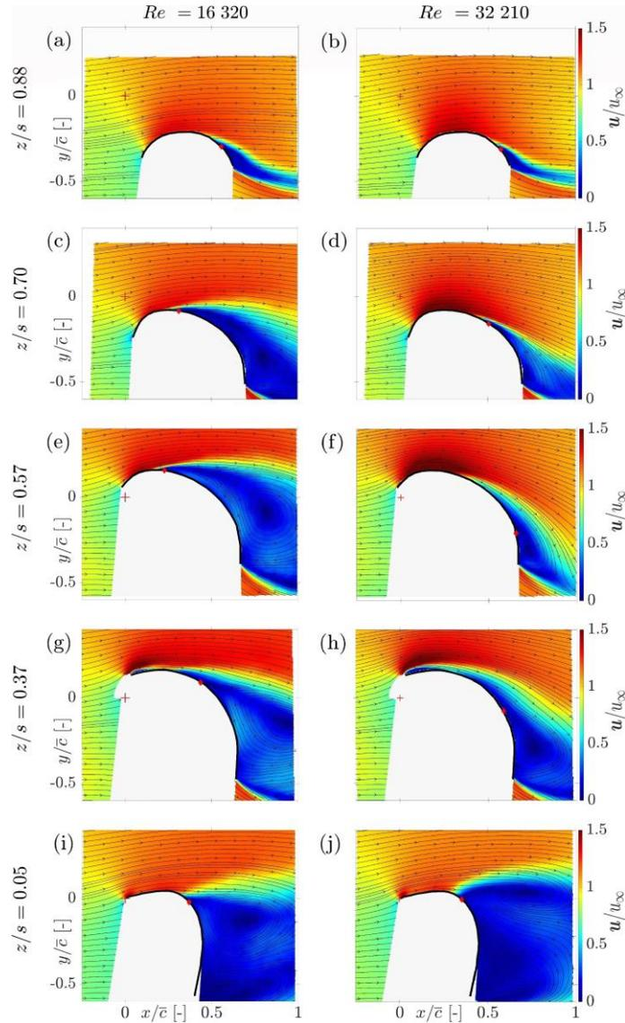
**Figure 11.** Streamlines and contours of nondimensional flow velocity for the 3D at  $\eta = 0^\circ$  for  $Re = 16\,320$  (left) and  $Re = 32\,210$  (right). Red diamond denotes the separation point.
