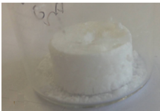
Figure 16: Photograph of shrinkage in SA/AG 1% (prepared as 1 TMOS: 2.4 TEB: 4.832 H 2 O: 10 -6 HCl: 10 -5 NH 4 OH and AG 1%, equ. 5) due to sublimation of TEB from inside the sol-gel formation at 0.3 mBar after it had been frozen at -10 °C. The measurement before drying were H= 25 mm and D= 28 mm, which shrunk to 14.5 mm and 24 mm, respectively, after drying.
