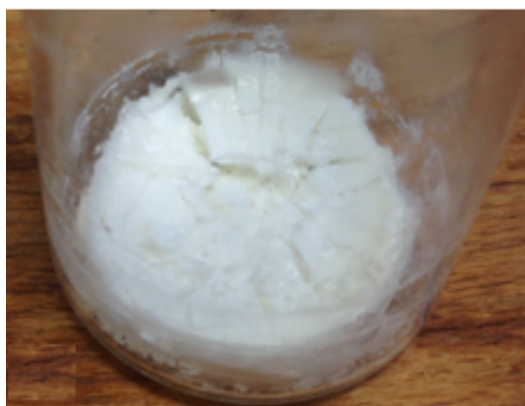
Figure 24: Photograph of SA/EC 5% prepared as 1 TMOS: 2.4 TEB: 4.832 H 2 O: 10 -6 HCl: 10 -5 NH 4 OH: 5*10 -3 EC (equ.9) by sublimation of TEB from inside the sol-gel formation at 0.2 mBar after it had been frozen at -10 °C. Before drying with 2.5 ml, D=28 mm and H=6 mm. After drying, H=4.4 mm and D=22 mm.
