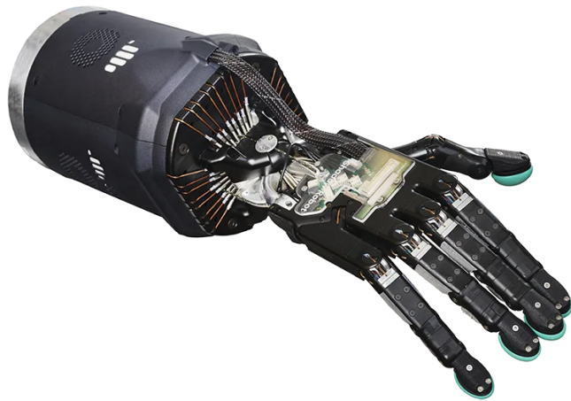
Figure 1.1: A commercialised anthropomorphic robot hand (Shadow Hand [93]). Picture from Shadow Robot company website: https://www.shadowrobot.com/
