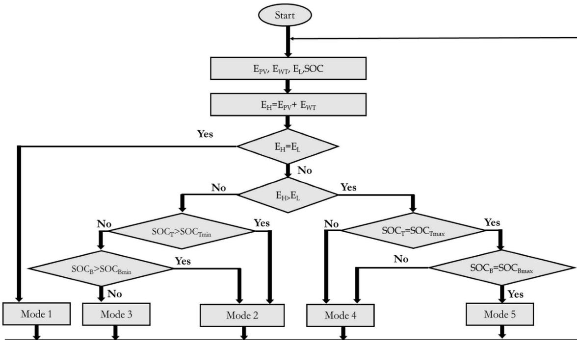
Fig. 2. Modes of operation of the hybrid energy system.
