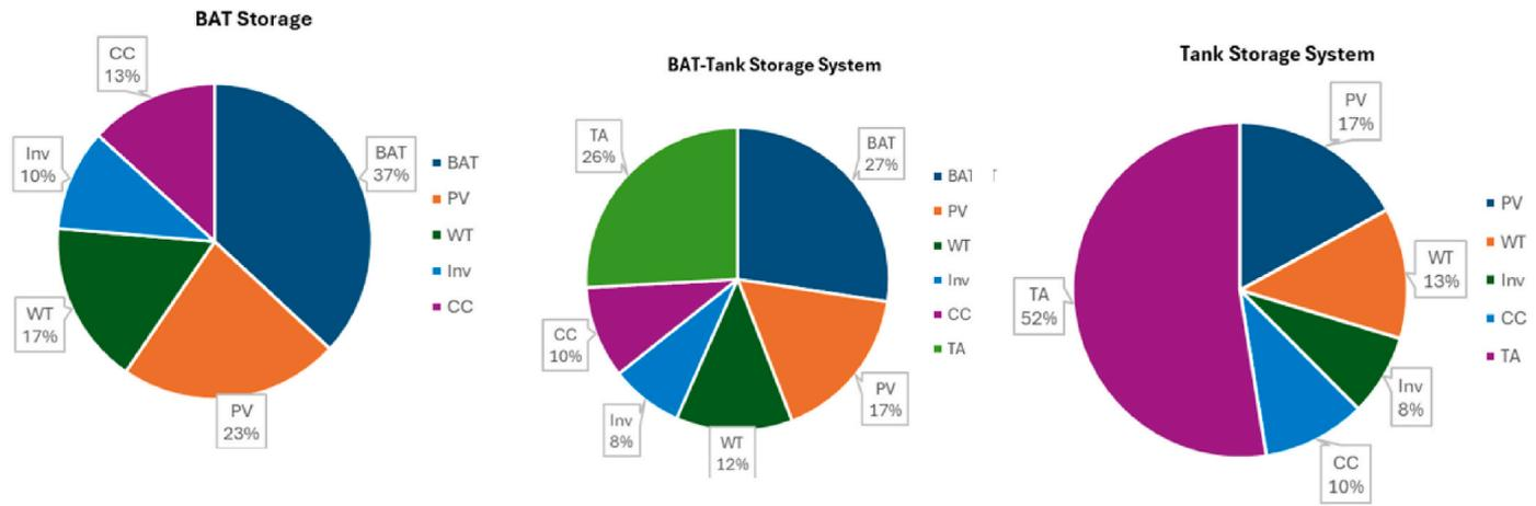
Fig. 13. Cost distribution a. Battery based system (left), b. Battery-tank based system (center), and c. Tank only storage system (right).
