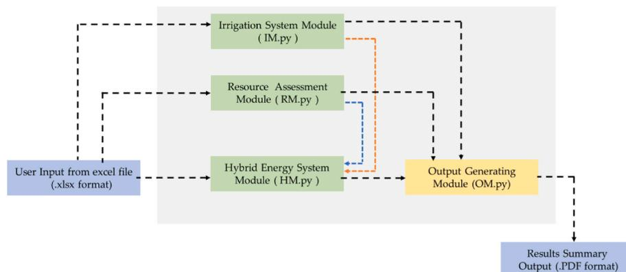
Fig. 3. System level model of the hybrid energy system.
