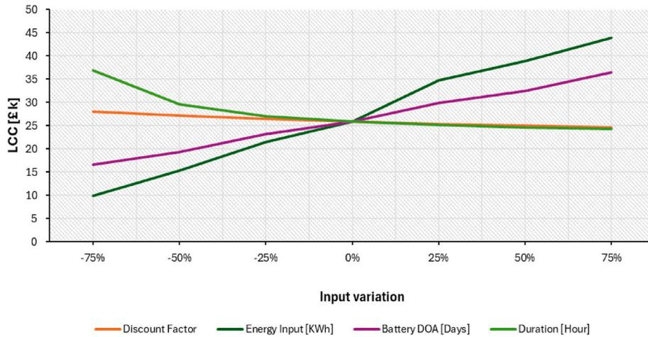
Fig. 4. Sensitivity study of various input variables in hybrid energy system.
