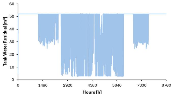
Fig. 12. Hourly water residual in the tank of battery-tank storage system.
