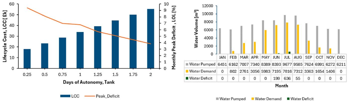
Fig. 8. a. Sensitivity analysis of LCC and LOLP (left), b. Monthly water pumped, water demanded and deficit (right) of tank only storage system.
