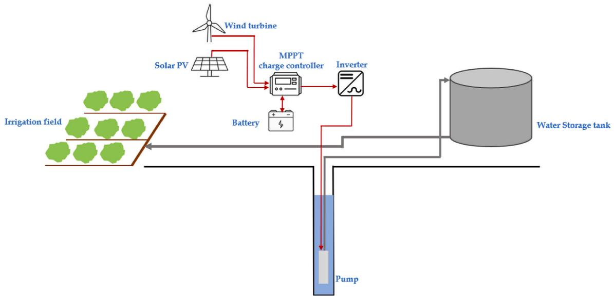
Fig. 1. Hybrid energy model block diagram.
