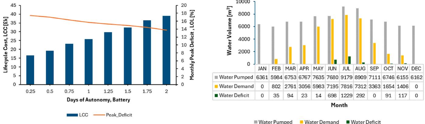
Fig. 6. a. Sensitivity analysis of LCC and LOLP (left), b. Monthly water pumped, water demanded and deficit (right) of battery only storage system.
