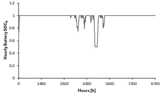
Fig. 11. a. Hourly water deficit (left); b. Hourly state of charge of the battery of battery-tank storage system.
