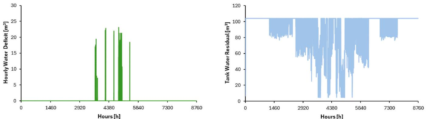
Fig. 9. a. Hourly water deficit (left), b. Hourly water residual in the tank (right) of tank only storage system.
