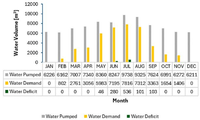
Fig. 10. a. Sensitivity analysis of LCC and LOLP (left); b. Monthly water pumped, water demanded and deficit (right) of battery-tank storage system.
