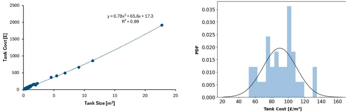
Fig. 5. a. Tank cost based on market study (left), b. Probability distribution of tank cost/m<sup>3</sup> (right).
