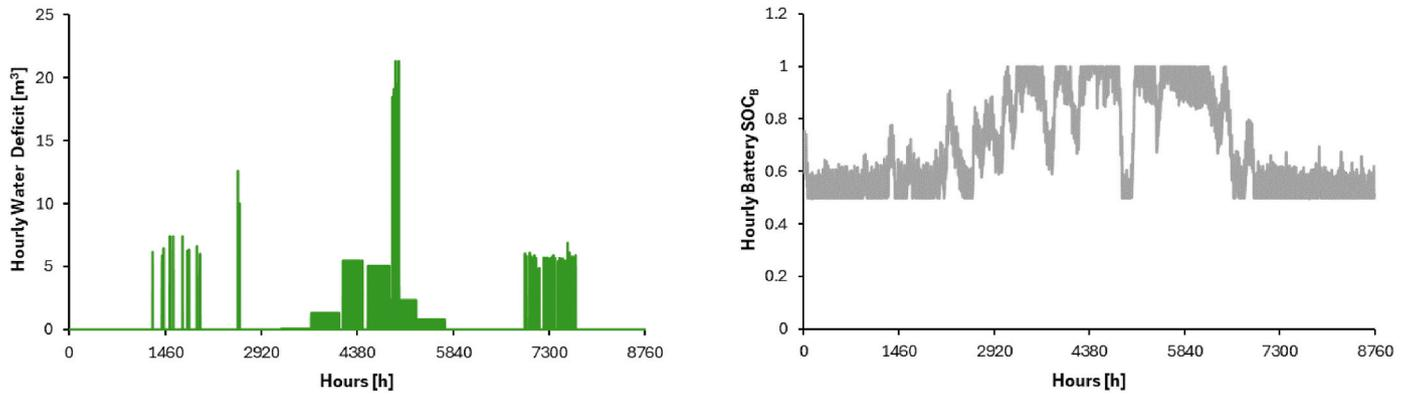
Fig. 7. a. Hourly water deficit (left), b. Hourly state of charge of the battery (right) of battery only storage system.
