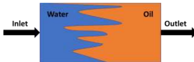
Figure 2.2: Viscous fingering effect: Water finger formation in the reservoir during water flooding.
